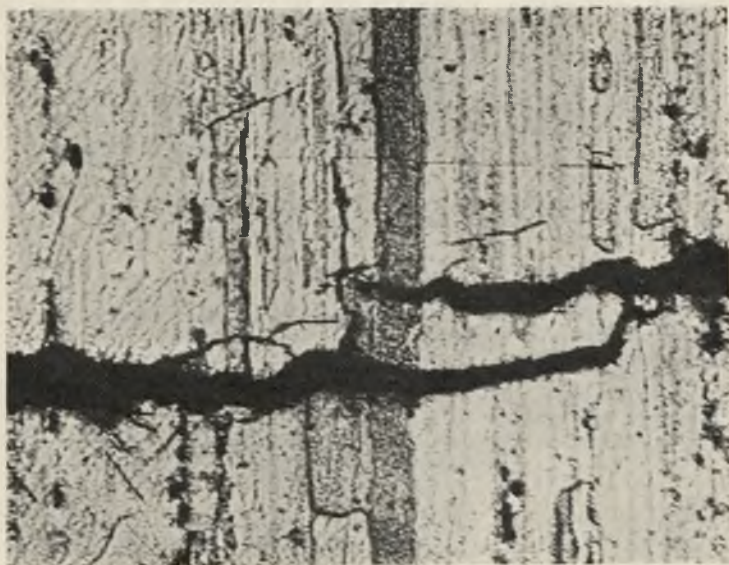
FIG. 6.—Section from Broken Fatigue Test-Piece, Etched. \times 200
