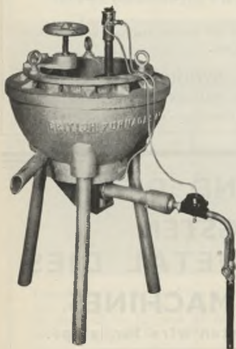
“PERFECTA” Temperature Regulator fitted to a Gas-fired Lead Melting Pot
