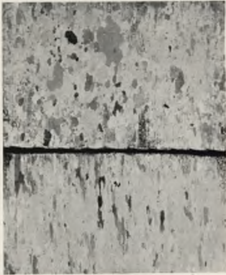
FIG. 11.—(Above) Equi-Axed Grains Usually Found in Tin Alloys. (Below) Elongated Grains in Copper-Tin Alloy. (0.45% Copper. Annealed at 222° C.)
