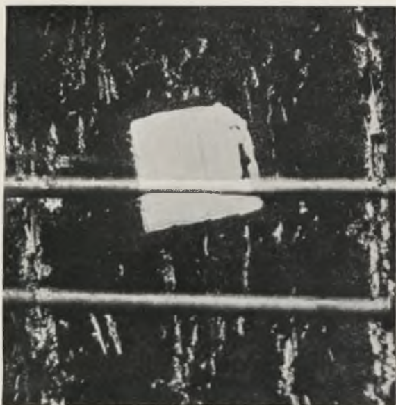
FIG. 4.—Scratch Tests on Babbitt No. II. \times 75 .
