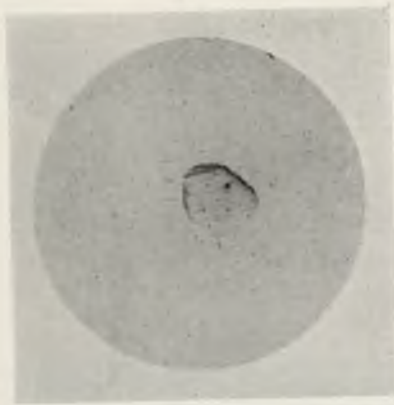
FIG. 3.—0.005% Nickel. Annealed at 228° C. for 7 days and Quenched. \times 1000 .
