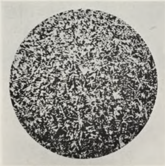
FIG. 23.—Alloy No. 2 + 1% Cadmium. Casting Temperature 450° C. Mould Temperature 18° C. \times 100 .
