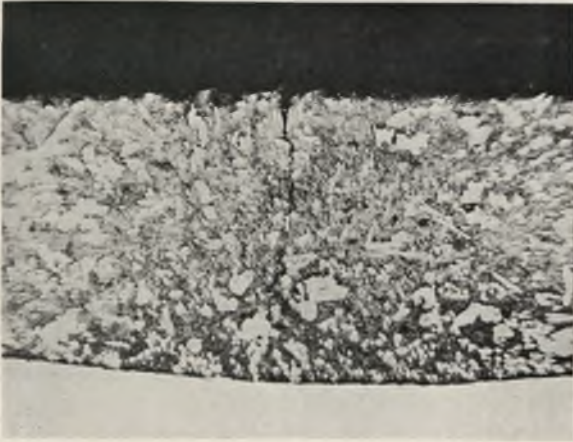
FIG. 5.—Cross-Section of a Cracked White Metal Coating, Showing a Typical Radial Crack. \times 50 .
