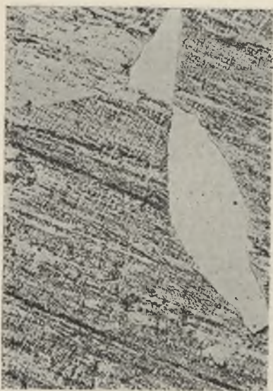
FIG. 7.—Alloy 42.3 Annealed for 5 Days at 462° C. White \gamma in grey (visually pink) \beta' . \times 150 .
