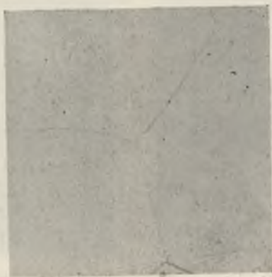
FIG. 15.—1% Cadmium. \alpha_1 only. \times 500 .
