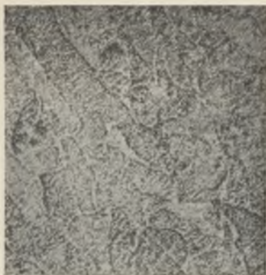
FIG. 7.—5% Cadmium. \alpha only. Annealed 3 Days. \times 500 .
