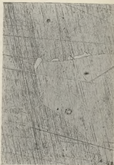
FIG. 8.—Alloy 51.8. Annealed at 586° C. Intergranular \alpha (white) in \beta . \times 150 .
