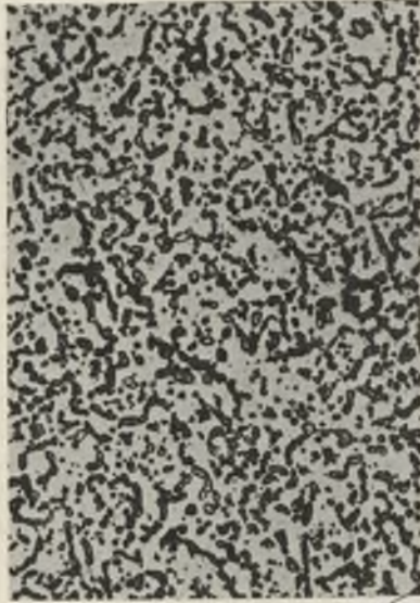
FIG. 4.—Alloy 46.8 Annealed until Uniform \beta' and Slowly Cooled to 224° C. Small \gamma crystals in \beta' ; primary \gamma is absent. \times 150 .
