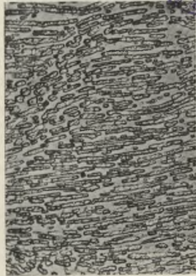
FIG. 6.—Alloy 45.3 Annealed until Uniform \beta' and Slowly Cooled to 224° C. Widmanstätten structure of \gamma in \beta' . \times 500 .
