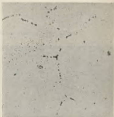
FIG. 8.—6% Cadmium. \alpha + Eutectic. Annealed 3 Days. \times 200 .
