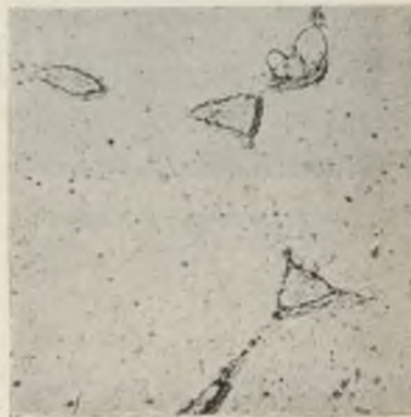
FIG. 12.—99.5% Cadmium. \beta + \alpha . Annealed 7 Days. \times 500 .
