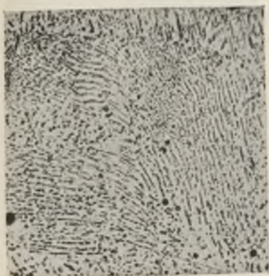
FIG. 13.—5% Cadmium. Eutectoid of White \alpha_1 and Dark \beta . \times 500 .
