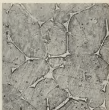
FIG. 22.—95% Cadmium. Quenched from 173° C. Dark \beta + Light \alpha . \times 200 .
