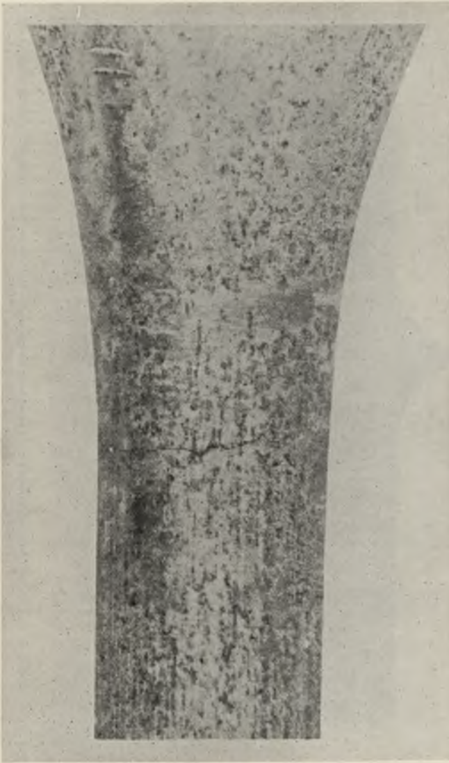
FIG. 11.—Specimen M15 (Unprotected Duralumin Tested in Salt-Spray) Showing Fatigue Crack after 8.09 million cycles of \pm 3.60 tons/in. 2 Stress. \times 6 .
