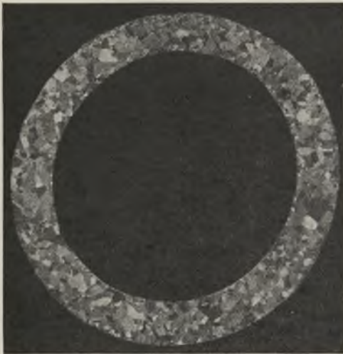
FIG. 6.—Lead Sheath used in Tests Recorded in Figs. 3-5. Section Showing Grain-Size. \times 2\frac{1}{2} .
