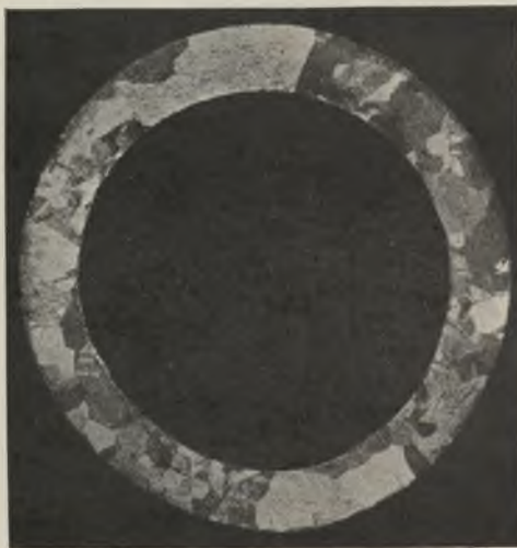
FIG. 7.—Lead Sheath Annealed 20 Hrs. at 250^{\circ} C. Section Showing Grain-Size. \times 2\frac{1}{2} .
