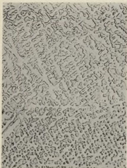
FIG. 8.— A_3M_3S_6 . As Cast. Typical Duplex Structure of this Series. \times 150 .
