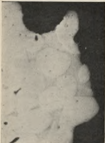
FIG. 3.—Section of Nickel-Chromium Wire, Showing Diffusion of Gold. Gold-Rich Phase is Dark. Unetched. × 500.
