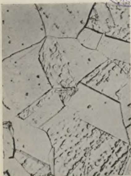
FIG. 2.—3M as Quenched from 900° C. Deeply Etched. \times 500 .
