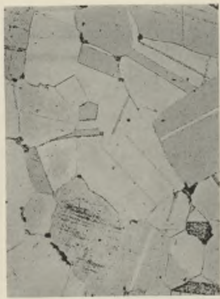
FIG. 7.— M_8S_5 . Annealed at 800^\circ C . for 30 Minutes. \times 150 .
