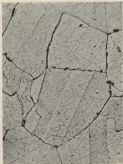
FIG. 8.—3M Slowly Cooled from 900° C. Etched. × 500.
