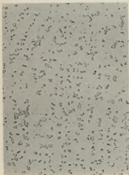
FIG. 14.— Si_2Sn_5 . As Cast. \times 150 .
