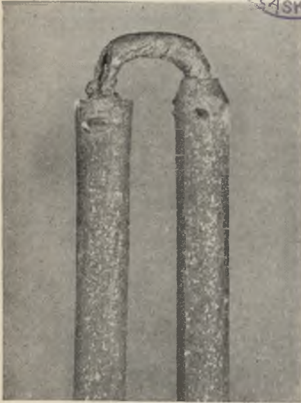
FIG. 1.—Gold Link Showing Partial Fusion. × 3.
