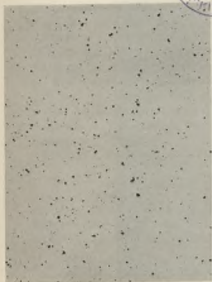
FIG. 12.— Fe_4S_{13} . Iron Particles Etched in 1% Nitric Acid in Alcohol. \times 150 .
