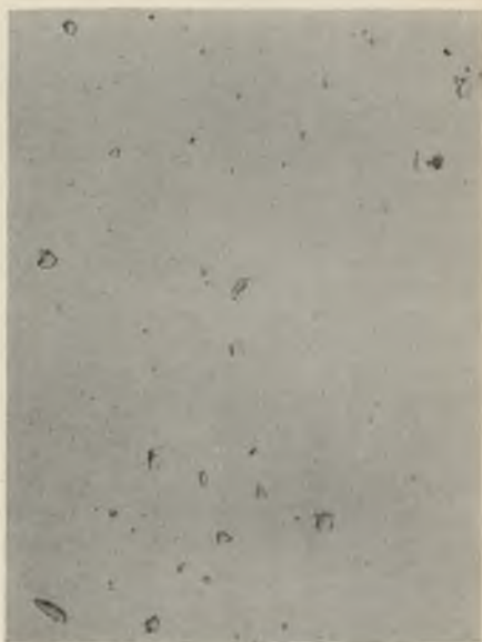
FIG. 18.— \text{Si}_3\text{Sn}_5 . Particles seen in Fig. 17. Annealed, Unetched. × 250.
