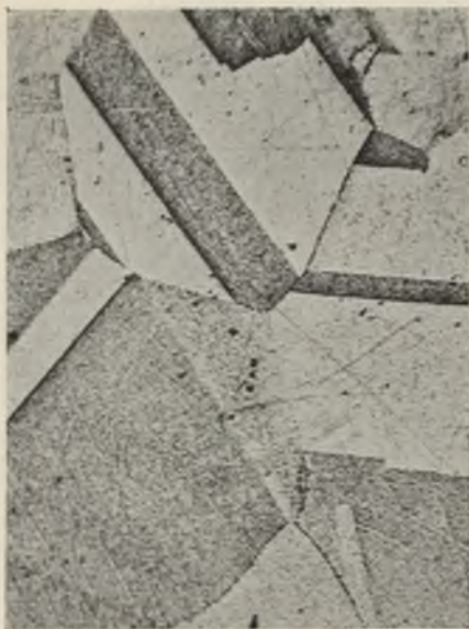
FIG. 6.—3M Quenched 900° C. and Re-Heated 1½ Hrs. 650° C. Etched. × 500.
