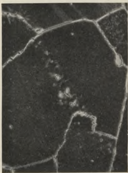
FIG. 9.—5P Slowly Cooled from 900° C. Etched. × 500.
