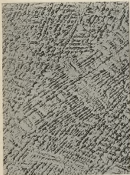
FIG. 6.— M_8S_5 . "As Cast" Structure after 15% Reduction. \times 150 .
