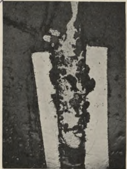
FIG. 2.—Section of Gold Link and Nickel-Chromium Wire, Showing Disintegration. Unetched. × 10.
