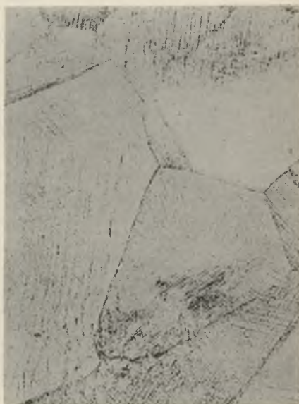
FIG. 9.— A_2M_3S_5 . Annealed at 800^\circ C. for 1 Hr. \times 150 .
