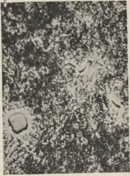
FIG. 11.—5P Slowly Cooled from 900° C. Etched. \times 2000 .
