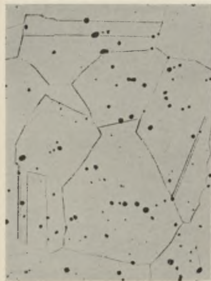
FIG. 10.— A_2M_2S_6 . Annealed at 800^\circ C. for 1 Hr. \times 150 .
