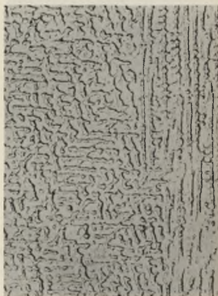
FIG. 11.— F_{10}S_5 . As Cast. Cored Solid Solution and Iron Particles. \times 150 .
