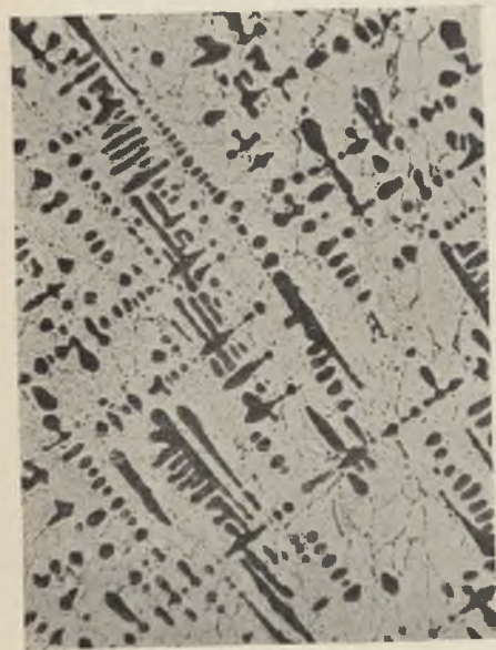
FIG. 12.—Alloy S Containing 20% Nickel + Silicon in Atomic Ratio 1 Ni/1 Si, Annealed 1 Week 700° C. and Quenched. Etched. \times 150 .
