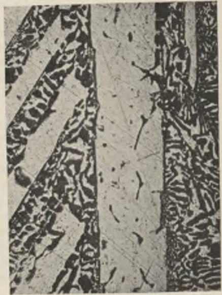
FIG. 13.—Alloy Y Containing 50% Nickel + Silicon in Atomic Ratio 2 Ni/1 Si, Annealed 1 Week 700° C. and Quenched. Unetched. \times 150 .
