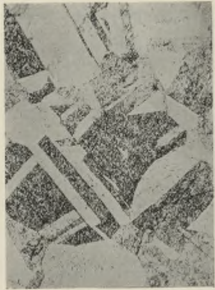
FIG. 4.— A_4S_5 . Annealed at 750^\circ C . for 12 Hrs. \times 150 .
