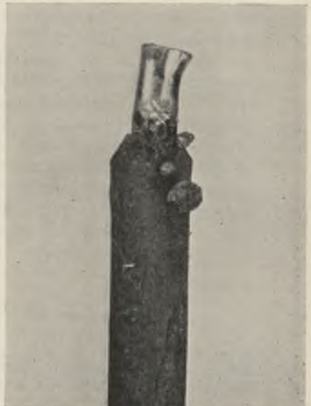
FIG. 4.—Experimental Test-Piece. 250 Hrs. at 950°–1000° C. in Air. × 5.
