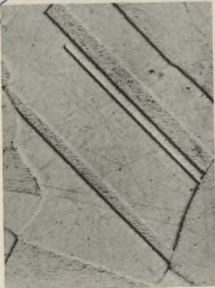
FIG. 3.—3M Quenched 900° C. and Re-Heated 1 Day 450° C. Etched. \times 500 .
