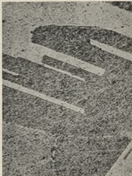
FIG. 7.—3M Quenched 900° C. and Re-Heated 1 Day 650° C. Etched. × 500.
