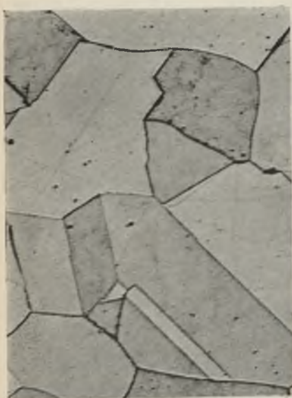
FIG. 4.—3M Quenched 900° C. and Re-Heated 22½ Minutes 540° C. Etched. \times 500 .
