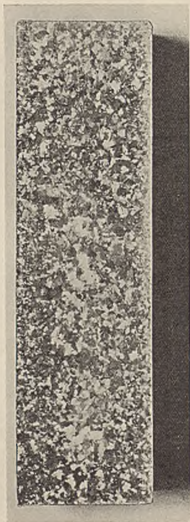
FIG. 14.—Section of Lead Beam Gauge-Length. Etched in Ammonium Molybdate.
