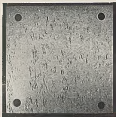
FIG. 11.—I.G. Process. 2 weeks' exposure.
