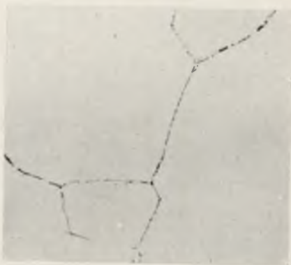
Fig. 4.—9.24 per cent. Aluminium quenched from 380° C. × 520.
