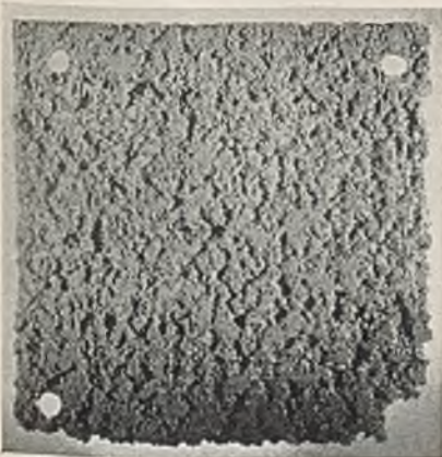
FIG. 5.—Jirotko Process. 8 weeks' exposure.
