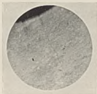
FIG. 2.—Duralumin Specimen Containing Fatigue Crack: After Polishing and Pickling Treatment D. \times 8 .
