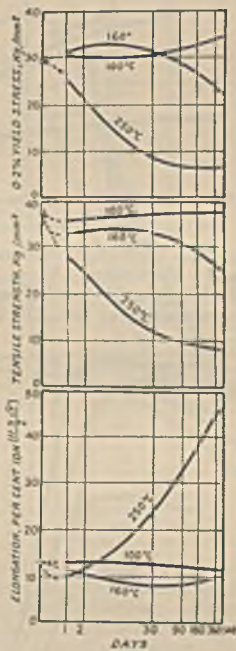
FIG. 26.—Influence of Continuous Heating at 100°, 160°, and 250° C. on Yield-Point, Tensile Strength, and Elongation of “R.R. 59” Alloy. Tested at 100°, 160°, and 250° C., Respectively.
