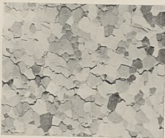
FIG. 13.—Intercrystalline Cracks in Creep Specimen. 1% Cadmium, Quenched and Tempered. \times 10 .
