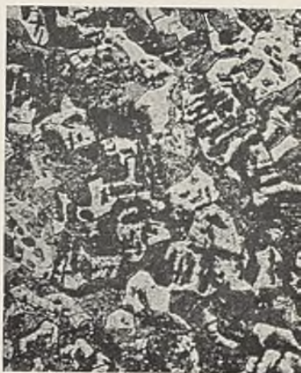
FIG. 13.—1.5% Cd. Quenched at 220° C. \alpha (light) + \beta (dark). \times 50 .
