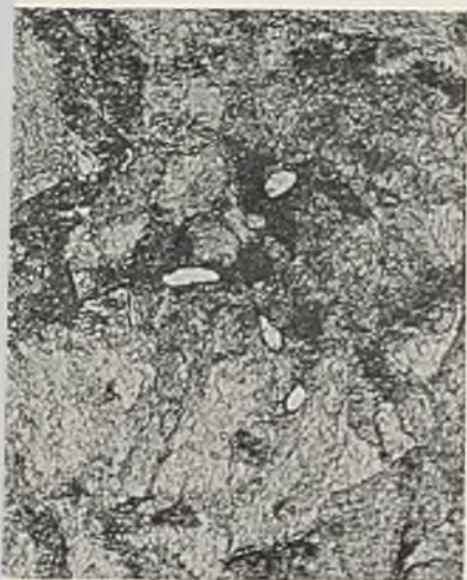
FIG. 12.—4.5% Cd. Quenched at 150° C. Traces of \alpha (light) in Decomposing \beta (dark). \times 400 .
