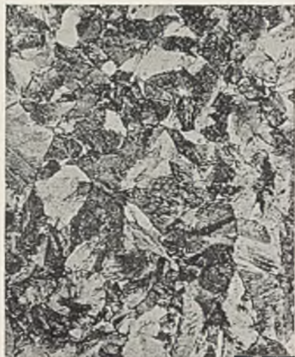
FIG. 9.—4.5% Cd. Quenched at 195° C. Recrystallized \beta . \times 100 .
