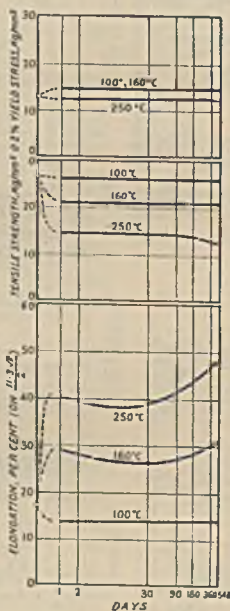
FIG. 22.—Influence of Continuous Heating at 100°, 160°, and 250° C., on Yield-Point, Tensile Strength, and Elongation of Peraluman 2. Tested at 100°, 160°, and 250° C., Respectively.
