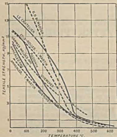
FIG. 1.—Tensile Strength of Pure Aluminium as Depending on the Temperature. Tested at the Annealing Temperature.
