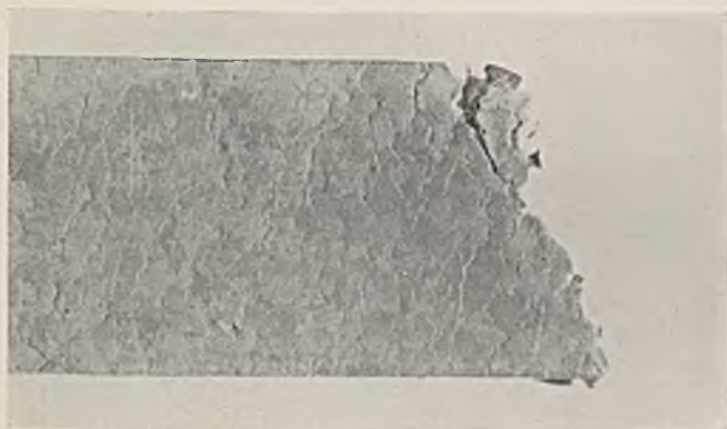
FIG. 11.—Creep Fracture. 1% Cadmium, Quenched and Tempered. \times 3 .
