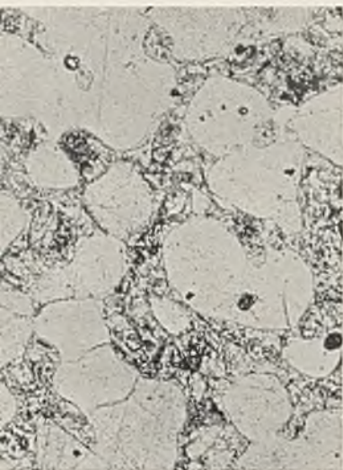
FIG. 8.—2% Cd. Quenched at 160° C. (white) + Recrystallized \beta (half tone). \times 200 .
