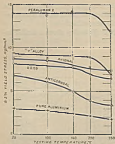
FIG. 27.—Yield-Point of Pure Aluminium and Aluminium Alloys Completely Stabilized as Depending on the Testing Temperature of 20°-250° C.
