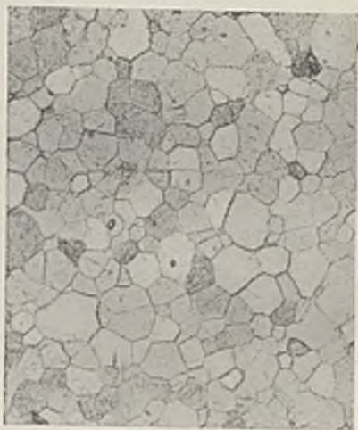
FIG. 5.—3% Bi. Etched Electrolytically in Dilute Hydrochloric Acid. \times 150 .
