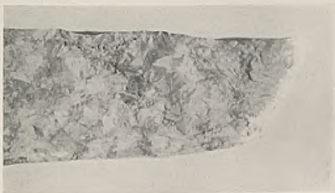
FIG. 12.—Tensile Fracture. 1% Cadmium, Quenched and Tempered. \times 3 .
