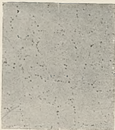
FIG. B.—Electrodeposited Chromium Annealed in Hydrogen for 10 Minutes at 1000° C.
