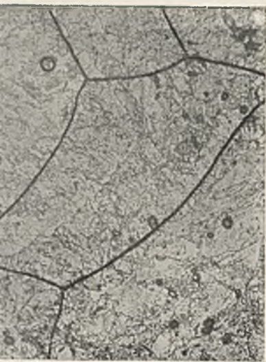
16.—3.5% Cd. Quenched at 210° C. crystallized \beta + Quenched Liquid (dark). \times 50 .
