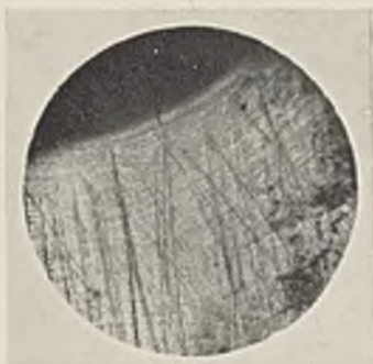
FIG. 1.—Duralumin Specimen Containing Fatigue Crack: Before Polishing and Pickling. \times 8 .
