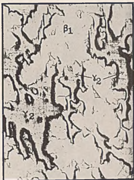
FIG. 30.—Sn 40, Hg 30, Ag 30%. Unetched. × 150.
