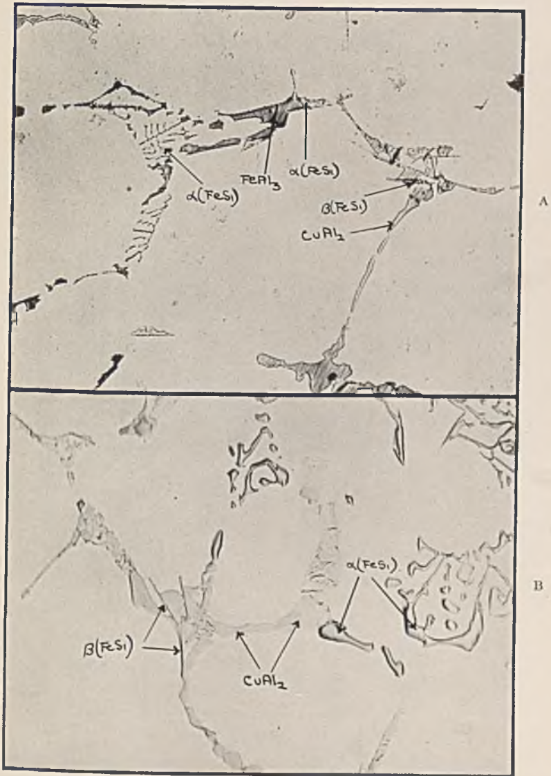
FIG. A.—Alloy "A" (Cu 5, Si 0.3, Fe 1 Per Cent.) Slowly Cooled in Furnace. Etched with NaOH. \times 300 .
