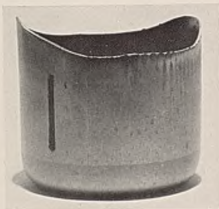
FIG. E.—Ears Formed in Brass Cup on One 45° Plane, with Wrinkles on the Other 45° Plane, Relative to Direction of Rolling (Marked with Thick Line).
