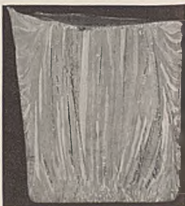
FIG. 10.—Two Halves of Ingot Machined; A, Vertically; B, Horizontally. \times \frac{1}{2} . FIG. 11.—Etched Axial Faces of Ingot Shown Above. \times \frac{1}{2} .
