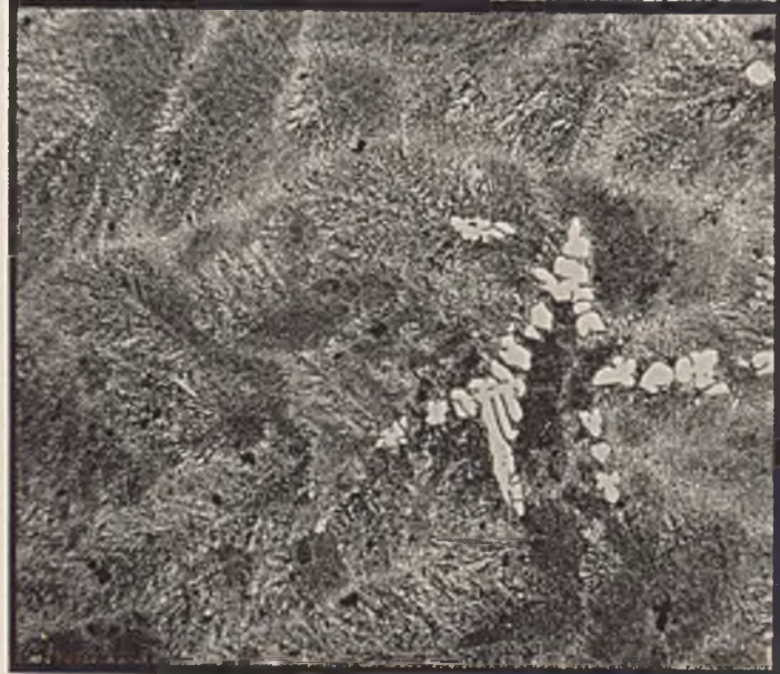
FIG. 7.—18.6% Cerium, As Cast. Etched in Citric Acid, Nitric Acid, and Glycerine. \times 150 .
