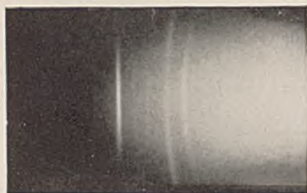
NOT ANNEALED SHOWING PREFERRED ORIENTATION (110) PLANE IN THE SURFACE
