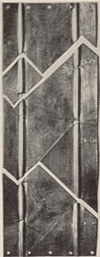
FIG. A.—Cross-Rolled Molybdenum Sheet Showing 45° Brittleness. \times \frac{1}{2} .
