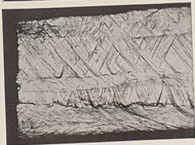
FIG. 12.—Loaded Zinc Test-Piece under Oblique Illumination; Surface Rippling Due to Twinning; Crystals Longitudinal. \times 3 .
