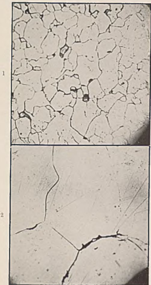
FIG. 1.—Brittle 75:25 Copper-Nickel. Unetched. \times 500
