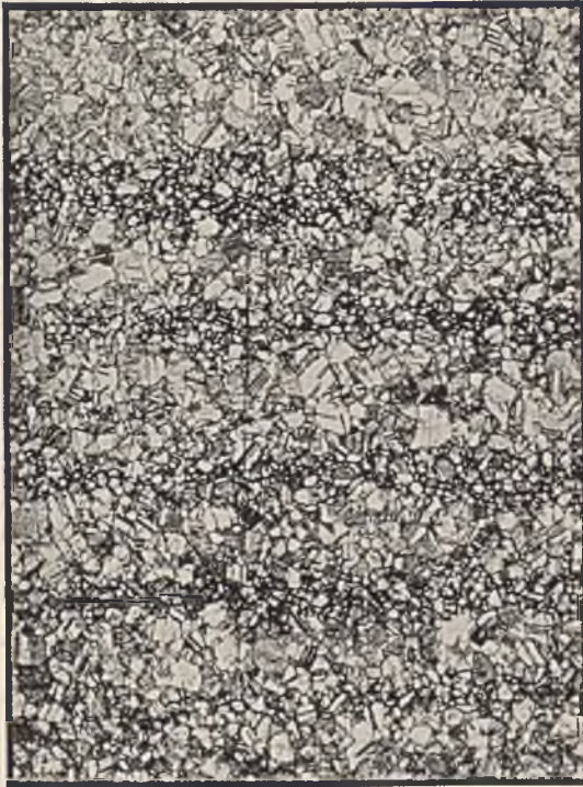
FIG. B.—Stringers of Small Crystals, Accompanied by \beta Particles, in Brass Sheet of Approximately 64% Copper Content. \times 75 .
