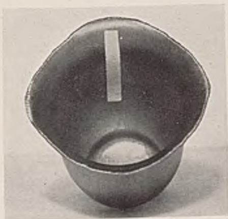
FIG. F.—Ears Formed in Steel Cup at 0° and 90° to the Direction of Rolling (Marked with Thick Line).
