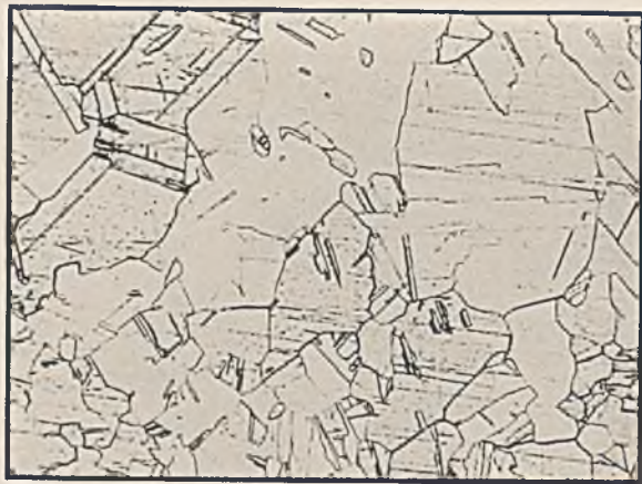
E. E. Fine Silver. Annealed (As Received). \times 100 .
