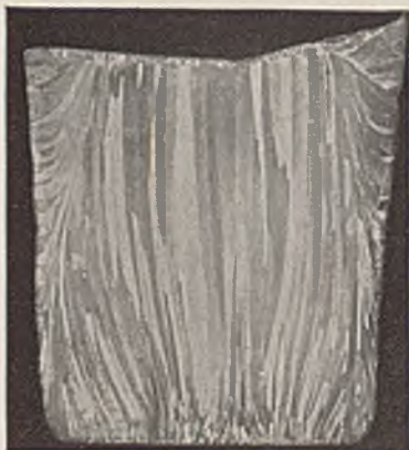
FIG. 10.—Two Halves of Ingot Machined; A, Vertically; B, Horizontally. \times \frac{1}{2} . FIG. 11.—Etched Axial Faces of Ingot Shown Above. \times \frac{1}{2} .
