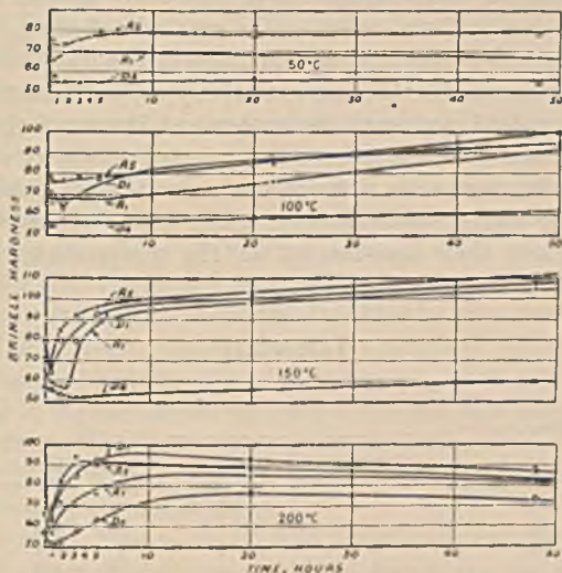
FIG. 6.—Forged Sand-Cast Bars Heat-Treated for 20 Hrs. at 500° C., Quenched in Water at Room Temperature and Then Aged at the Temperatures Given.
