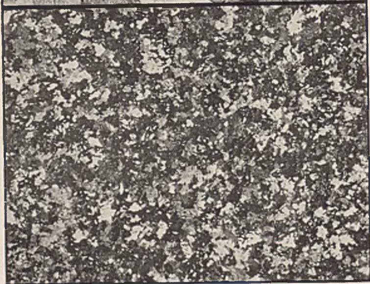
FIG. 21.—Grain Growth in Service. Intercrystalline Cracking. \times 2 Diam. FIG. 22.—Recrystallized Structure. \times 5 Diam.
