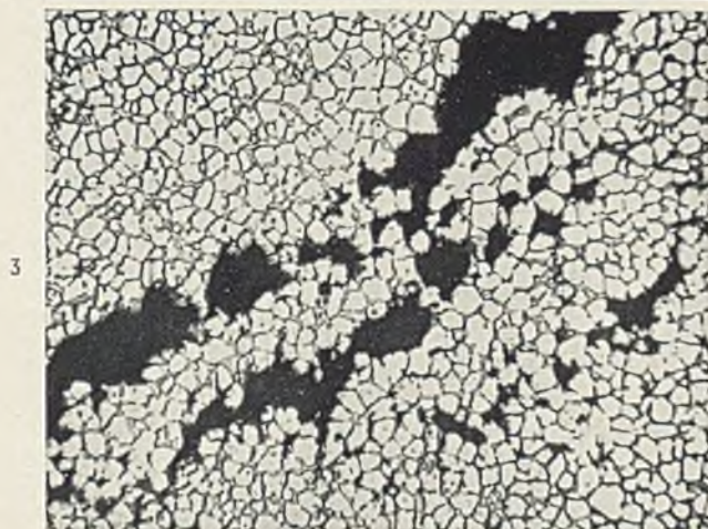
FIG. 1.—Hair-Line Cracks in Cast Alloy Revealed by Machining.
