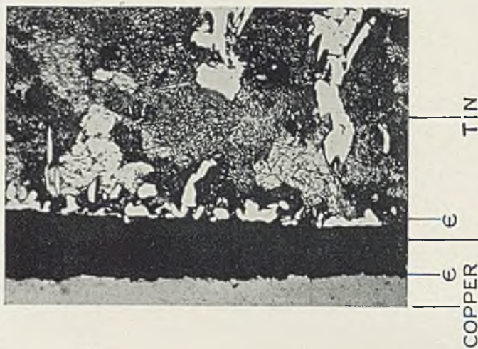
FIG. 10.—Pure Tin and HC. Copper. 30-Second Joint Fractured. Strength 11 lb./in. \times 500.
