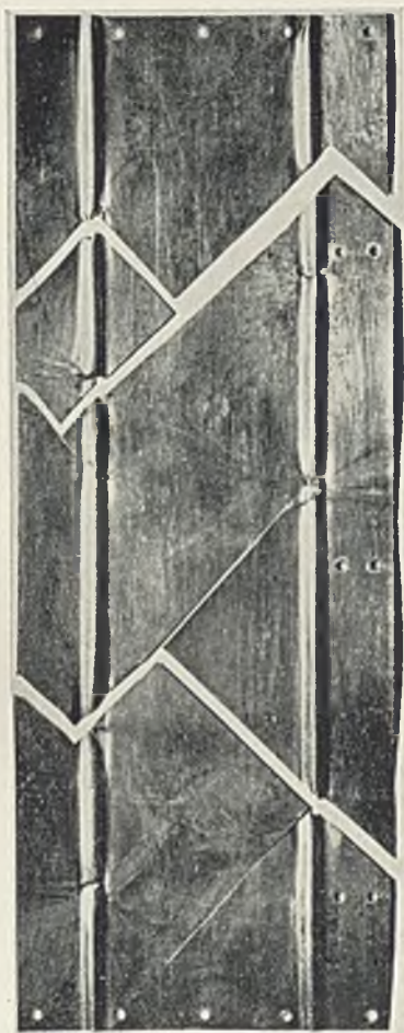
FIG. 1.—Sample of Cross-Rolled Molybdenum Sheet Showing 45° Brittleness. (Natural Size.)
