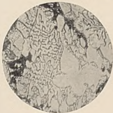
FIG. 11.—Cu 30, Mg 1%. FIG. 14.—Cu 30, Mg 8%.
