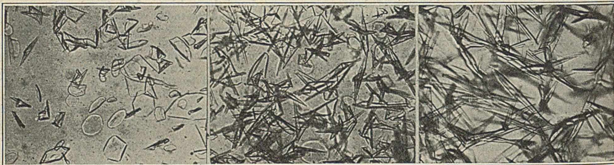
Figure 1—Initial stage of crystallization on slow cooling. Plate crystals beginning to curl at edges
