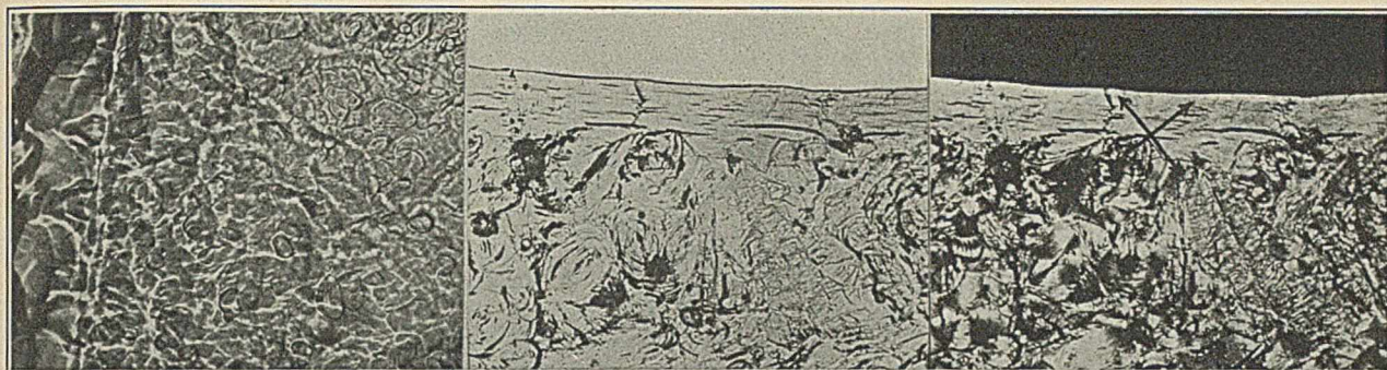
Figure 4—Wax that has been cooled very slowly, almost to complete solidification. Consists almost entirely of plates
