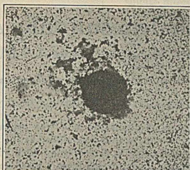
Figure 5—Armco iron corroded with water; corroding spot appeared after half an hour. 100 X
