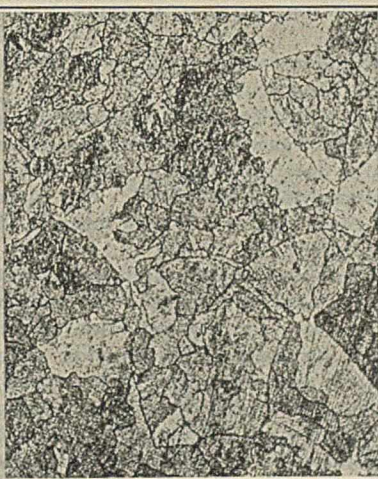
Figure 15—Lead-tin alloy, 3 per cent tin. Treated at 200^{\circ}\text{C} . for 1/2 hour and quenched. \times 100
