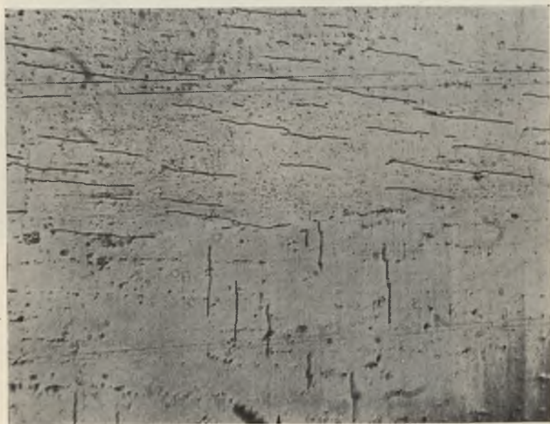
FIG. 19.—Specimen FKY5A. \lambda = 305^\circ . Cracks About Boundary 3, 5 (After Etching). \times 100 .
