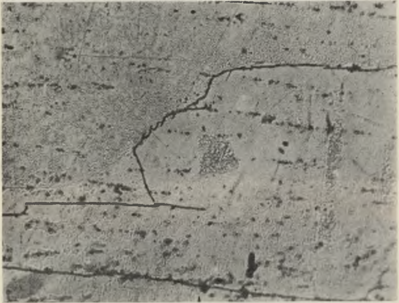
FIG. 20.—Specimen FKY1A. \lambda = 206^\circ . Part of Boundary 1, 2 (Shown in Fig. 21, Plate IX) (After Etching). \times 180 .
