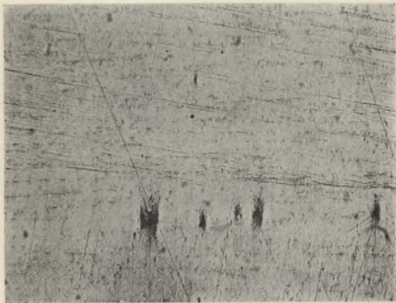
FIG. 7.—Specimen FKY1C. \lambda = 272^\circ . Slip at Boundary 4, 1. \times 100 .
