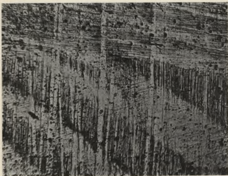
FIG. 11.—Specimen FKY5A. \lambda = 310^\circ . Part of Boundary 3, 5. \times 100 .
