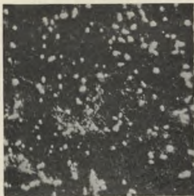
FIG. 8.—7% Antimony. Annealed at 190° C. White Precipitate of \delta in Dark \alpha . \times 300 .
