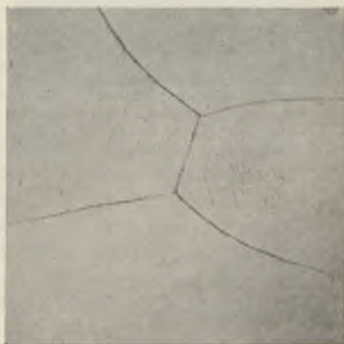
FIG. 12.—8% Antimony. Quenched from 230° C. \alpha . \times 50 .
