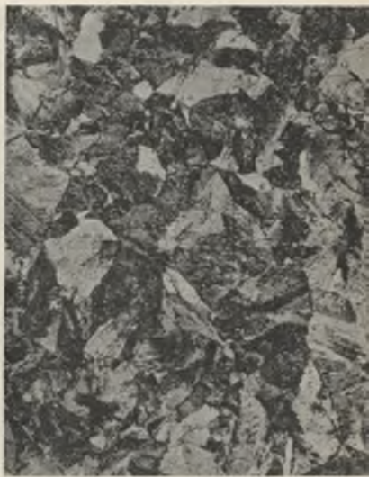
FIG. 9.—4.5% Cd. Quenched at 195° C. Recrystallized \beta . × 100.
