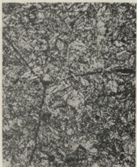
FIG. 15.—5.6% Cd. Quenched at 160° C. \beta + Intergranular \gamma . \times 400 .
