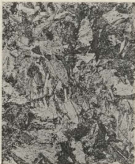
FIG. 10.—3.5% Cd. Quenched at 205° C. Recrystallized \beta . × 400.
