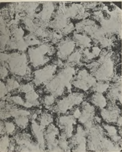
FIG. 4.—3.5% Cd. Slowly Cooled from Melt. Primary \alpha (light), Peritectic \beta (half tone), Traces of Eutectic (dark). \times 50 .
