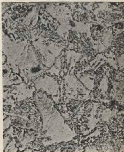
FIG. 17.—4% Cd. Heated Slowly to 140° C. Quenched Immediately. Formation of \alpha (light) from Eutectoid (matrix). \times 100 .
