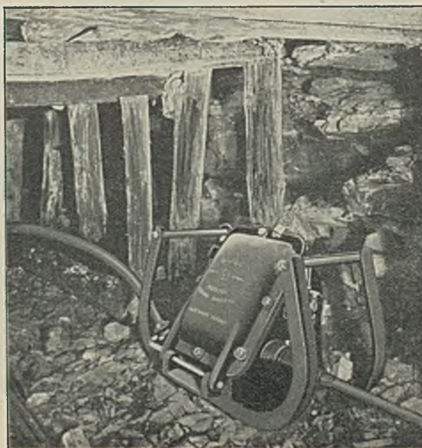
Fig. 12.—Circuit Breaker at the Gate-end.
