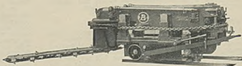
Fig. 3.—An Arcwall Electric Chain Machine with Elevating Gear: Jib raised. (Anderson, Boyes & Co., Ltd.)
