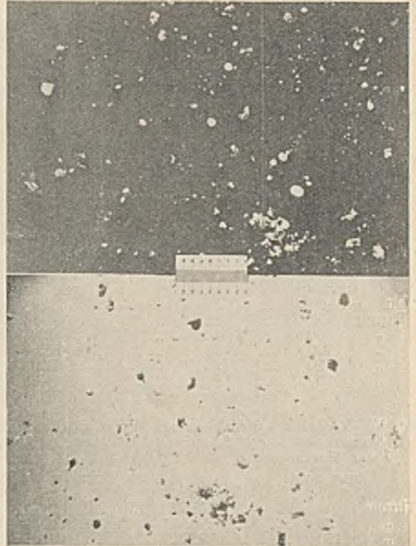
Fig. 6.—Ungraded dust from Pulverised-fuel-fired Water-tube boiler fitted with Turbulent burners; photographed against light and dark background.
