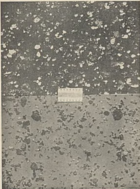
Fig. 4.—Ungraded dust from Pulverised-fuel-fired Water-tube boiler fitted with Calumet burners; photographed against light and dark background.
