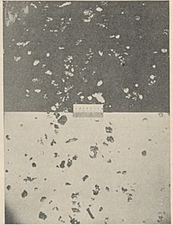
Fig. 5.—Ungraded dust from Pulverised-fuel-fired Water-tube boiler fitted with Fishtail burners; photographed against light and dark background.
