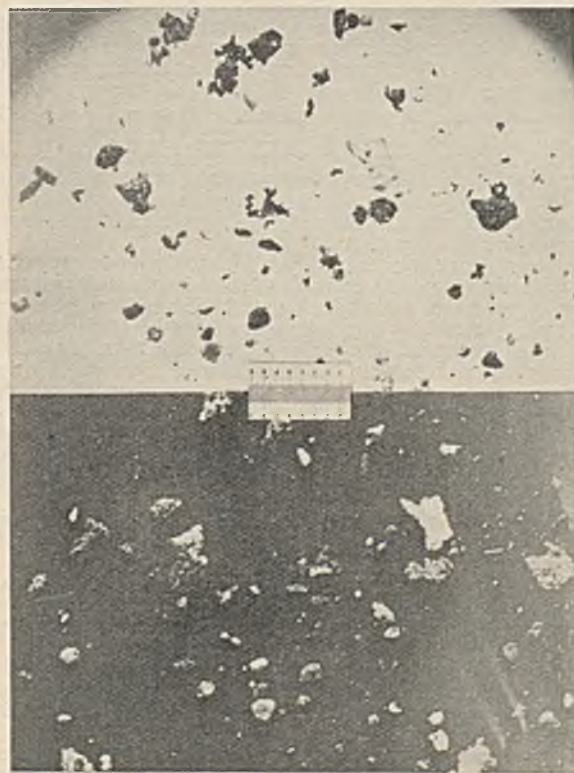
Fig. 2.—Ungraded dust from Stoker-fired Water-tube boiler; photographed against light and dark background.
