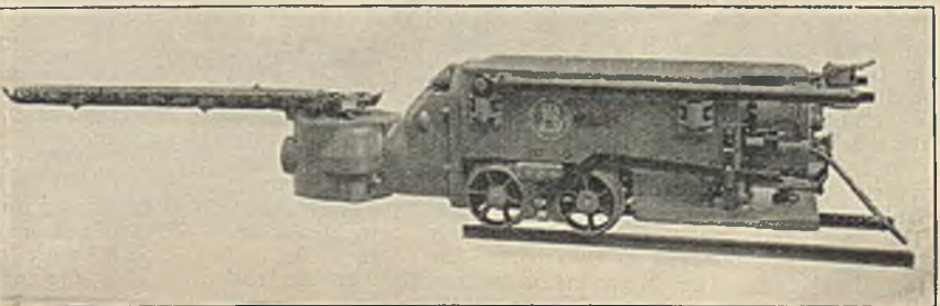
Fig. 5.—Jib in Highest Position for Holing as an Overcutter.
