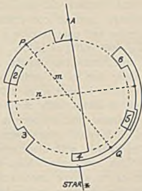
Fig. 7.—Method of reconnecting the rotor of a motor to ensure its retaining its central position by a corrective pull.
