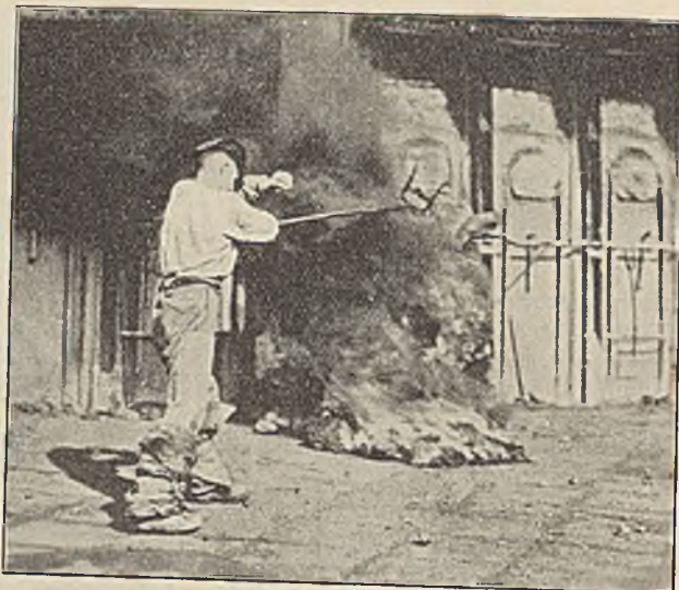
Fig. 8.—Old Method—Breaking Coke Cake.
