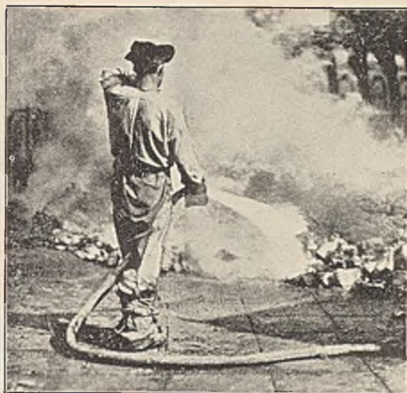
Fig. 10.—Old Method—Hose Quenching.
