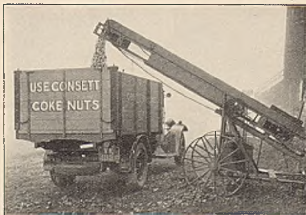
Fig. 23.—Portable Electric Conveyor-Loader.
