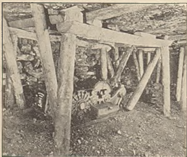
Fig. 12.—Electric Driving Gear for Shaker Conveyors connected to the end of the troughing. It may also be placed at the side of, underneath, or at right angles to the troughing (Mavor & Coulson).
