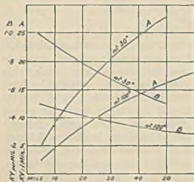
Fig. 1.—Varnished Cloth: Effect of Thickness on Breakdown Voltage.
