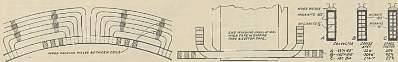
Fig. 13.—Details of A.C. Motor Stator Insulation.
