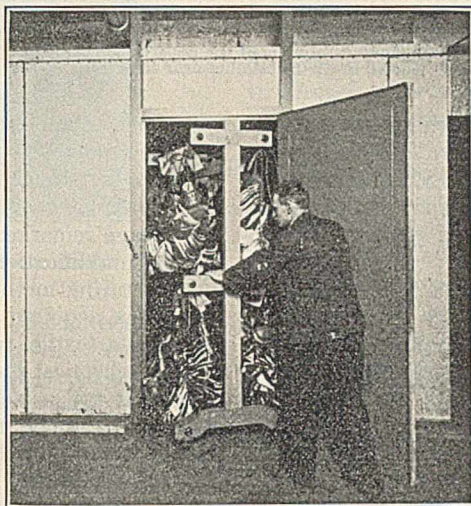
Subjecting of Shoe Uppers to Conditioned Air Prior to Stretching on Lasts. International Shoe Company
