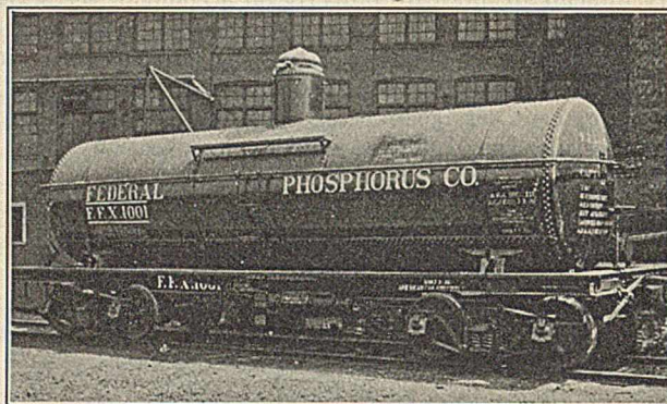
Figure 12—Rubber-Lined Tank Car for Transporting 85 Per Cent Phosphoric Acid
