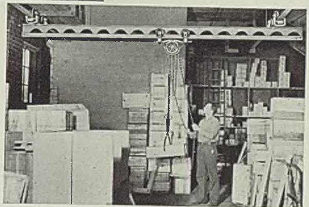
Two-runway cranes are available for capacities of 3 tons, 45-ft. span and 5 tons, 25-ft. span. Longer spans may be covered with cranes operating on three, four, and more runways.
