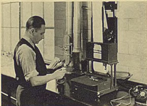
Samples of steel are delivered from melt shop to laboratory by compressed air and analyses reported to furnace department by telautograph system
