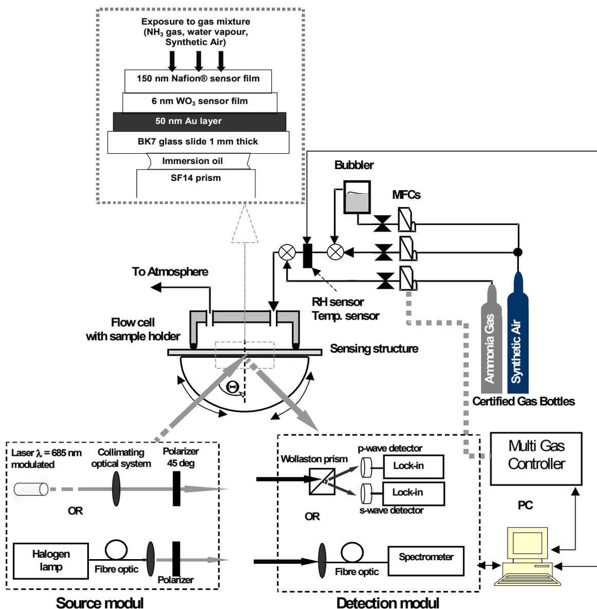
Fig. 3. The experimental set-up for measurements of variations in the optical signal of a light reflected from the sensor structures.
