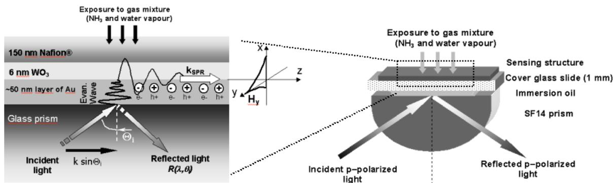
Fig. 2 Configuration of SPR sensor for ammonia gas detection.
