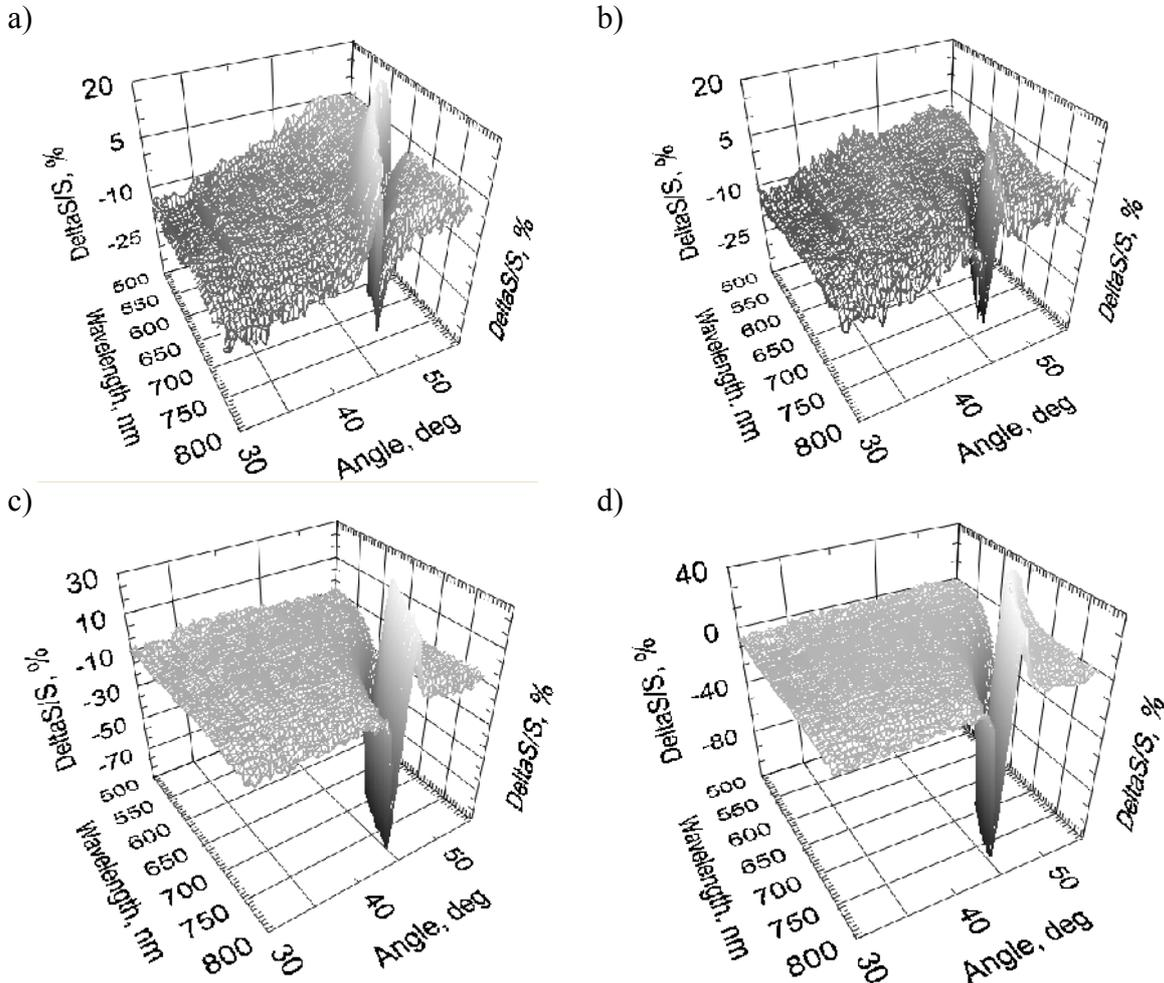
Fig. 6. Reflected light intensity change (in %) for the sensing structure as a function wavelength and angle of incident light for (a) RH 2% (dry air) (b) RH 48% (c) RH 60% (d) RH 83%. Structure was exposed to gas mixture flowing with 500 ml/min rate and consisting water vapour.
