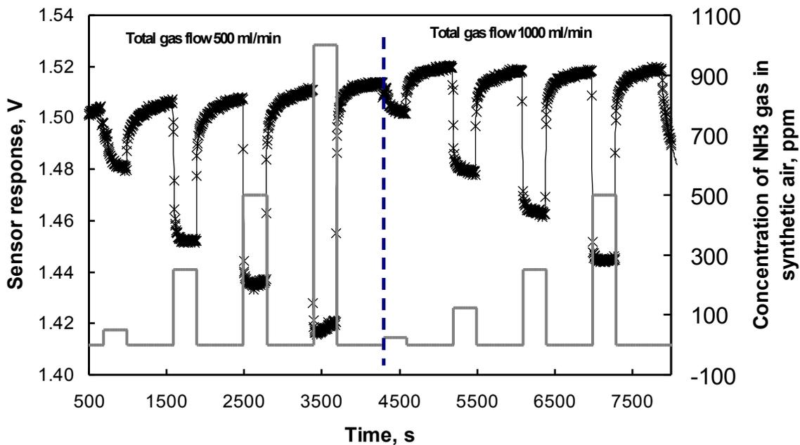
Fig. 4. The optical signal variation of the SPR sensor versus the time exposition varying concentrations of  $\text{NH}_3$  at room temperature and dry air. Experimental conditions: p-polarized monochromatic light  $\lambda = 685$  nm, incident angle of light  $\Theta = 49.2$  deg.
