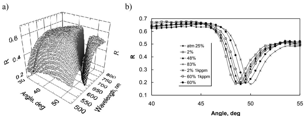
Fig. 5. Measured reflectance of sensing structure (a) as a function wavelength and angle of incident light for p-polarized light (air atmosphere RH 23%) and (b) for different concentrations of the water vapour and 1000 ppm of  $\text{NH}_3$  in dry and wet (RH 60%) air, 685 nm p-polarized light.
