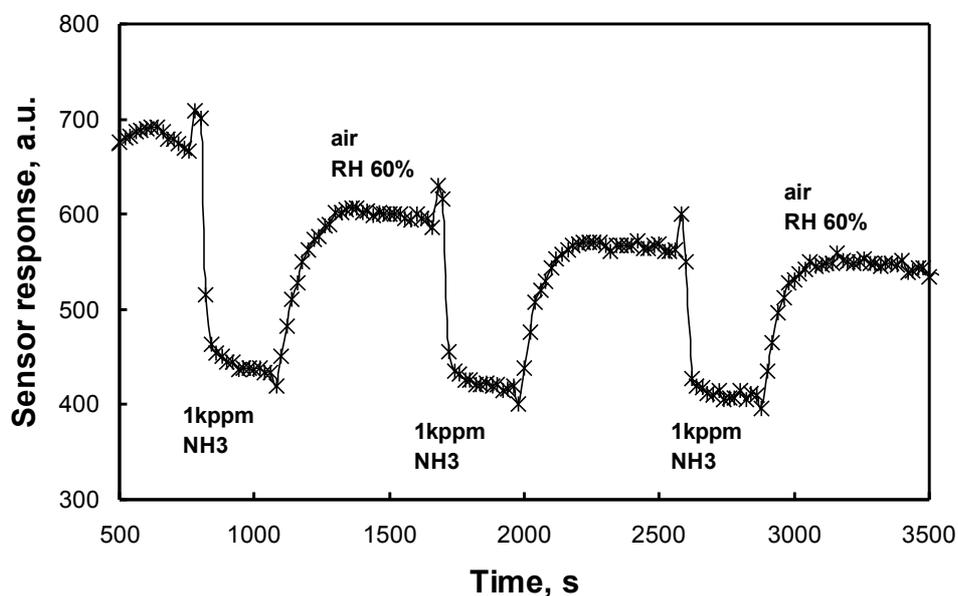
Fig. 7. The optical signal variation of the SPR sensor versus the time exposition varying concentrations of  $\text{NH}_3$  at room temperature and humid air (60% RH). Experimental conditions: p-polarized monochromatic light  $\lambda = 685$  nm, incident angle of light  $\Theta = 49.2$  deg.
