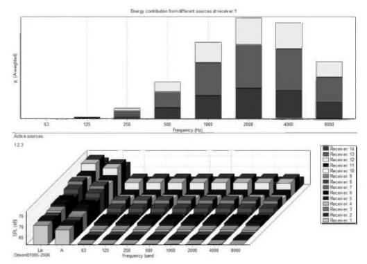
Fig. 9.4 The share of source energy in point 1 and sound level distribution at reception points for octave frequency bands
