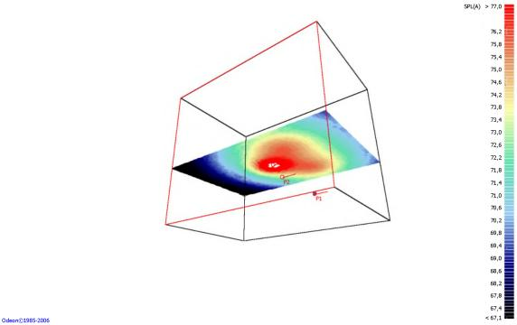
Fig. 9.3 Sound level distribution at reception points
