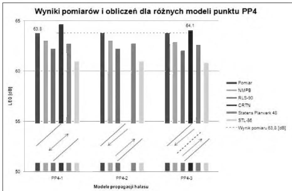
Fig. 2.8 Comparison of measurements' results and model calculations' results of noise emission from a district single carriageway road (point PP4)
