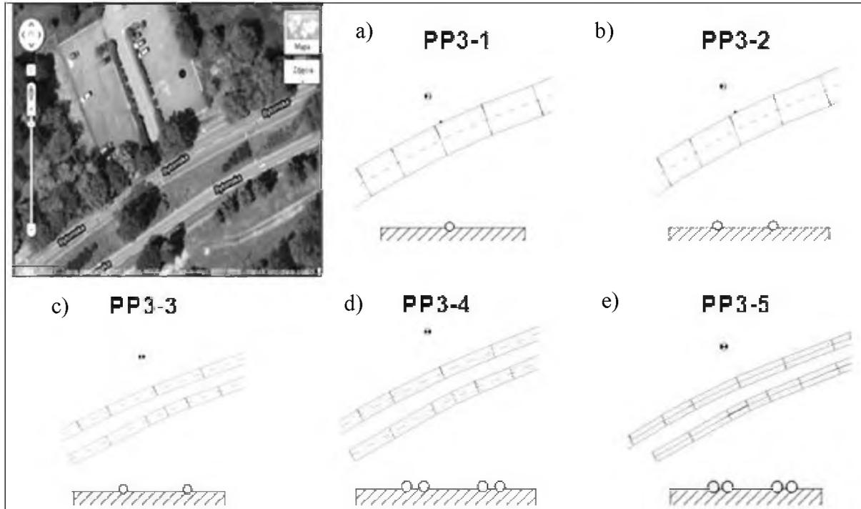
**Fig. 2.3 Exemplary models of the noise source for a dual carriageway road (point PP3):**
