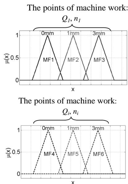
Fig. 10. System „II” of the rules construction system of fuzzy logic, MF1...6 – following appurtenance functions
