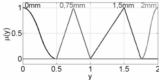
Fig. 7. Way number 1 of construction of the fuzzy outputs of the fuzzy logic system for a damage in the form of the chipping tip of the tooth
