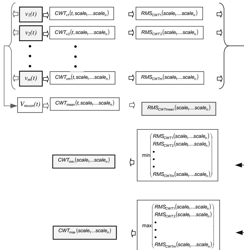
Fig. 4. The way a classifier model using fuzzy logic is built
