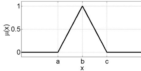
Fig. 5. A chosen input appurtenance function
