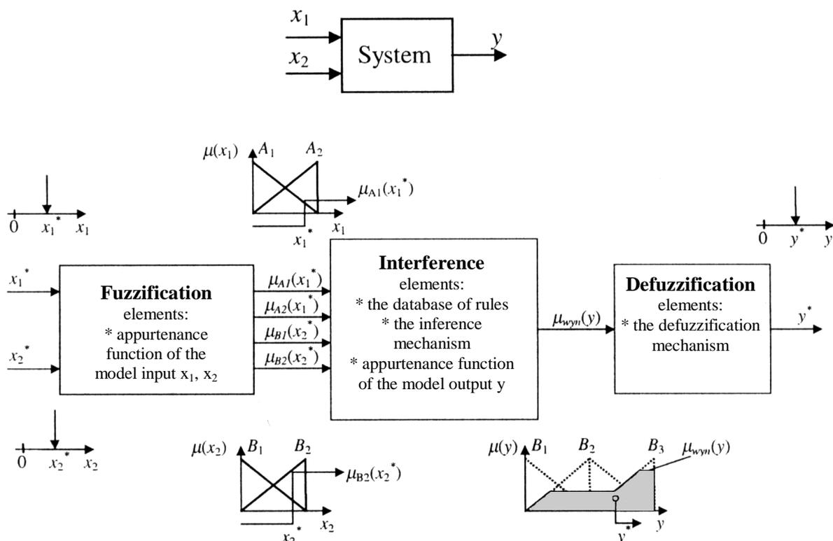
Fig. 1. The example structure of a fuzzy model
