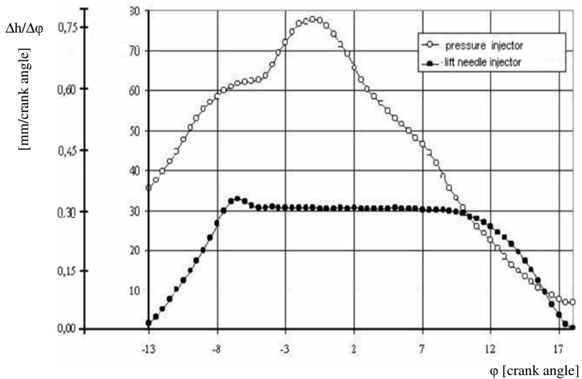
Fig. 4. The course of the injector needle lift speed and the injection pressure for the engine speed of 4250 [rpm]
