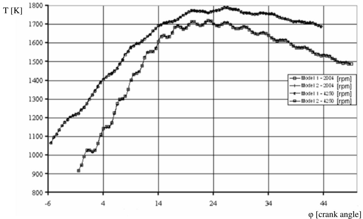
Fig. 5. The course of average combustion temperature for two engine speed
