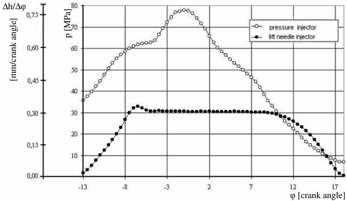
Fig. 3. The course of the injector needle lift speed and the injection pressure for the engine speed of 2004 [rpm]
