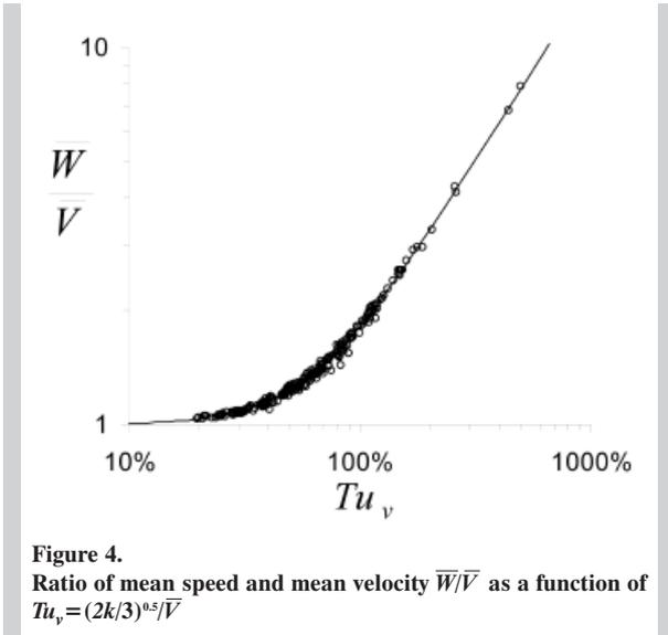
**Figure 4.** Ratio of mean speed and mean velocity  $\bar{W}/\bar{V}$  as a function of  $Tu_v = (2k/3)^{0.5}/\bar{V}$
