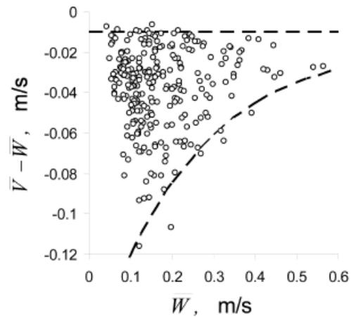
Figure 2. Difference between mean velocity  $\bar{V}$  and mean speed  $\bar{W}$ , based on the analyses of velocity measurement database performed by 3-D LDA in rooms under realistic conditions, Melikov (1997)
