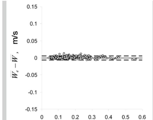
**Figure 5.** Difference between the estimated mean speed,  $\bar{W}_e$ , calculated by means of eq.6 (or 7), and the mean speed,  $\bar{W}$ , obtained from the analyses of LDA measurements. The dotted lines define the area with 95% of the measurement points
