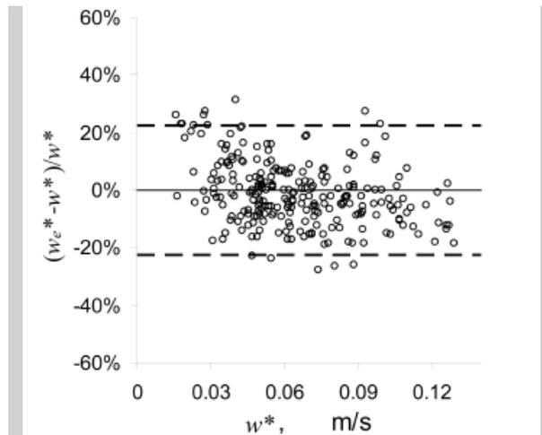
**Figure 6.** Relative difference between  $w_e^*$  (estimated standard deviation of speed, calculated from eq. 15) and measured speed standard deviation  $w^*$ , data from measurement performed by Laser Doppler Anemometer in rooms under realistic conditions, Melikov (1997)
