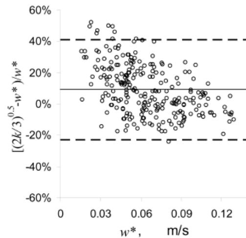
Figure 3. Difference between the standard deviation of velocity,  $(2k/3)^{0.5}$ , and the standard deviation of speed,  $w^*$ , based on the analyses of velocity measurement database performed by 3-D LDA in rooms under realistic conditions, Melikov (1997)
