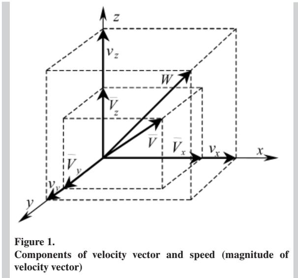
Figure 1. Components of velocity vector and speed (magnitude of velocity vector)
