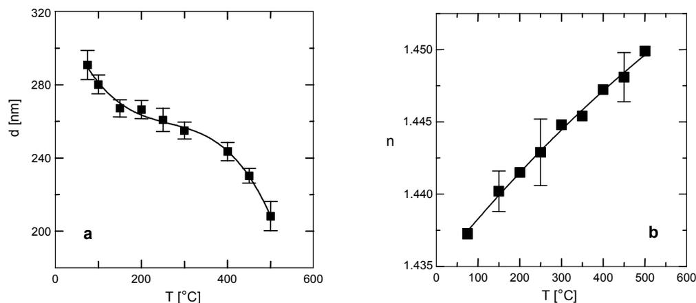
Fig. 8. Influence of annealing temperature: on the final film thickness (a), on refractive index (b).
