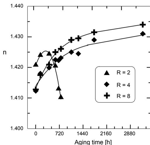
Fig. 3. Changes of refractive index of the films during their aging.
