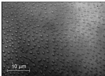
Fig. 4. Microscopic image of the structure after being aged for 1085 h in ambient conditions. Molar ratio TEOS:H<sub>2</sub>O:EtOH:HCl = 1:2:4:0.02.
