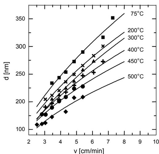
Fig. 7. Dependence of film thickness on the substrate withdrawal speed for different annealing temperatures.
