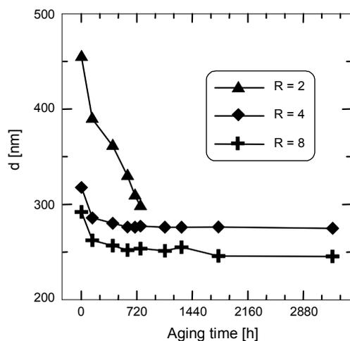
Fig. 2. Changes of thickness of the sol films during their aging for different water content  $R$ . Lines are drawn as guides for eye.
