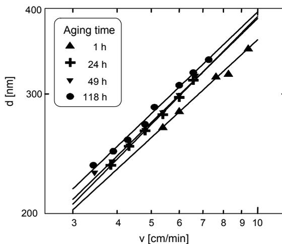
Fig. 1. Dependence of the thickness on the substrate withdrawal speed for different aging times of sol (TEOS:H<sub>2</sub>O:EtOH:HCl = 1:4:4:0.02).
