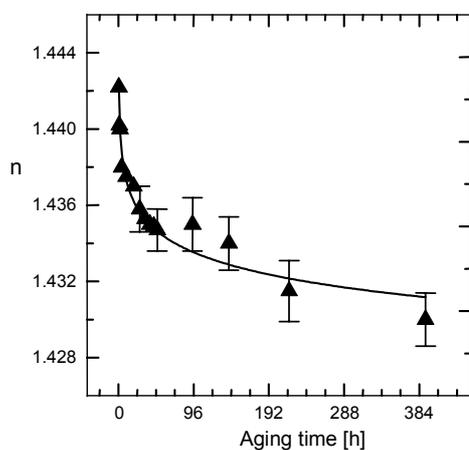
Fig. 5. Influence of aging time of the sol films on final refractive index. Films were aged at 18°C and relative humidity of 66% and then were annealed at 150°C for 2 h. Substrate withdrawal speed  $v = 5.0$  cm/min.
