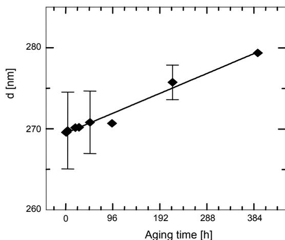
Fig. 6. Influence of aging time of the sol films on final thickness.
