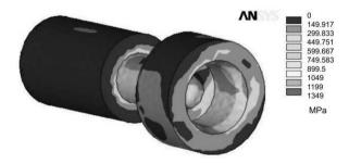
Fig. 6. Reduced stresses in the double threaded screw loaded with the force F = 2000 N
