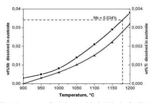
Fig. 5. Temperature dissolution (precipitation) kinetics for TiN ( $\blacktriangle$ ) and NbC ( $\blacksquare$ ) in austenite
