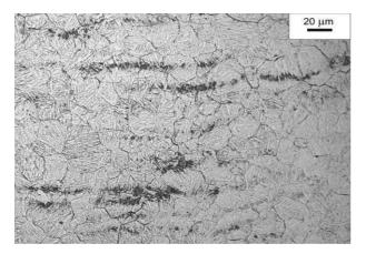
Fig. 3. Structure of primary austenite of the specimen water-quenched from a temperature of  $1000^{\circ}$ C
