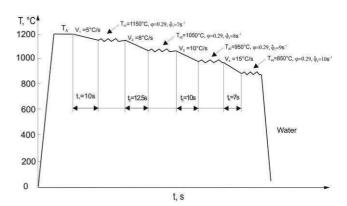
Fig. 1. Conditions of multi-stage hot-compression test
