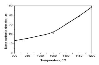
Fig. 2. Influence of austenitizing temperature on a grain size of primary austenite
