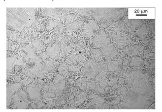
Fig. 4. Structure of primary austenite of the specimen water-quenched from a temperature of  $1100^{\circ}$ C
