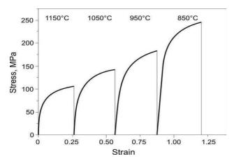
Fig. 8. Stress-strain curves corresponding to hot-working conditions in Fig. 1
