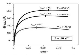
Fig. 7. Influence of temperature on stress-strain curves of the specimens compressed at a strain rate of  $10s^{-1}$
