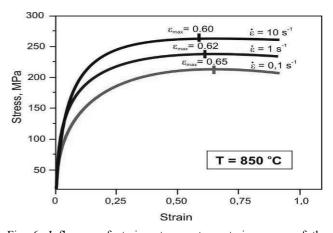
Fig. 6. Influence of strain rate on stress-strain curves of the specimens compressed at a temperature of 850°C
