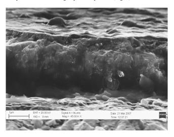
Fig. 4. Fracture surface of the gradient (Ti,Al,Si)N coating deposited onto the  $Al_2O_3+SiC_{(w)}$  oxide tool ceramic
