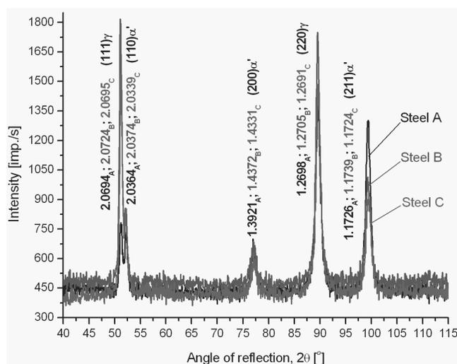
Fig. 9. X-ray diffraction patterns of steel grades A, B and C with a draft of 70%
