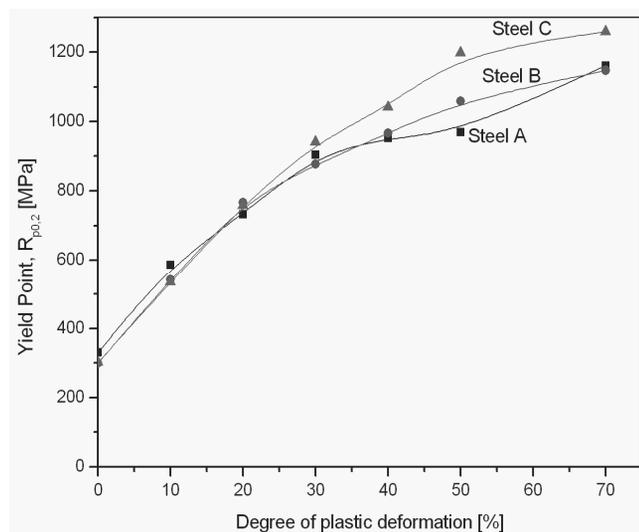
Fig. 3. Changes of the yield point investigated cold rolled steel A, B and C depending on degree of deformation
