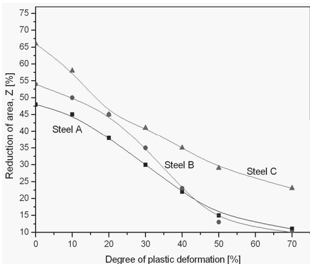
Fig. 6. Changes of the reduction of area in the investigated cold rolled steel A, B and C depending on the degree of deformation
