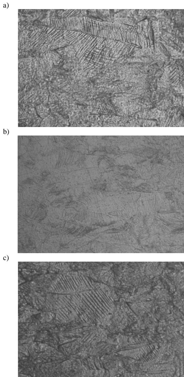
Fig. 2. Structure of the investigated steel type X5CrNi18-10 after deformation with a rolling reduction of 50%; a-c melts of these steel; Etching - Mi17Fe; Mag. 500x
