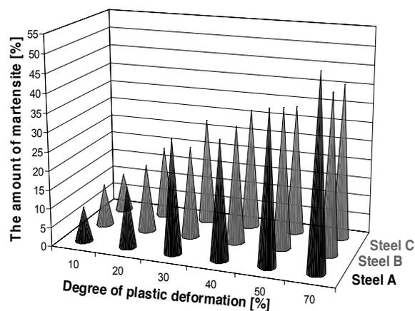
Fig. 8. Dependence of the volume fraction of  $\alpha'$ - phase on degree of plastic deformation investigated steel
