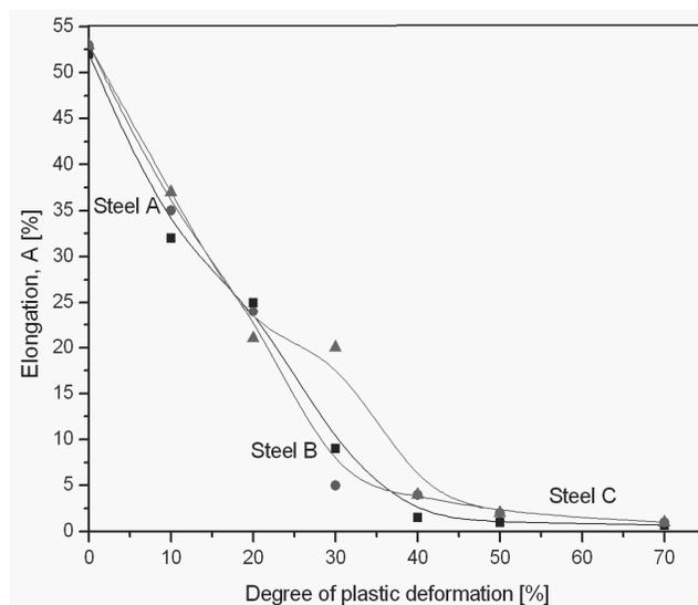
Fig. 5. Changes of the elongation investigated cold rolled steel A, B and C depending on degree of deformation
