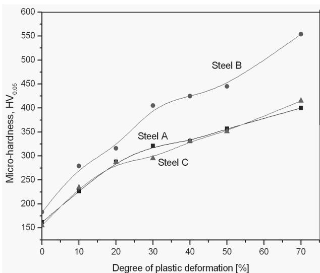
Fig. 7. Changes of the micro-hardness investigated cold rolled steel A, B and C depending on degree of plastic deformation
