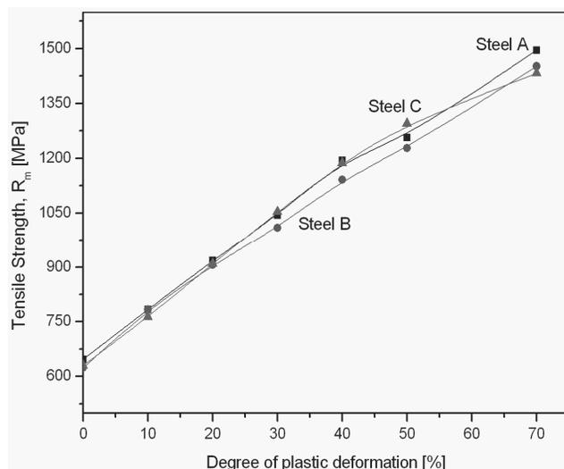
Fig. 4. Changes of the tensile strength investigated cold rolled steel A, B and C depending on degree of plastic deformation
