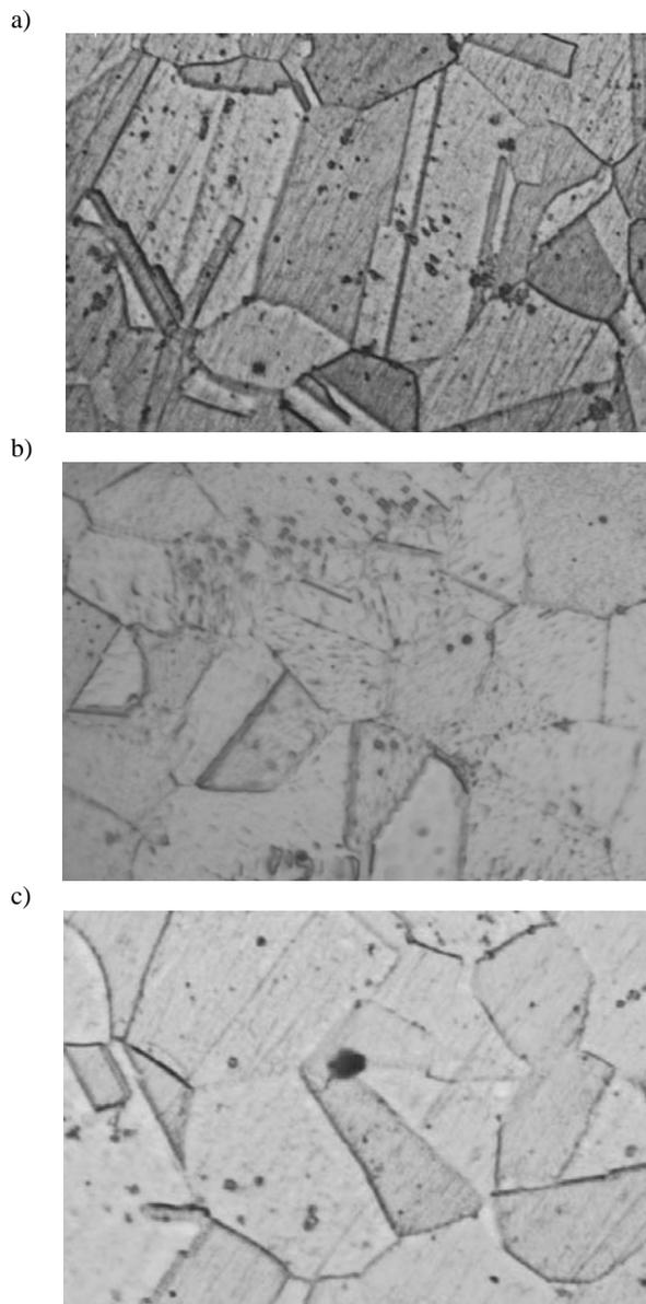
Fig. 1. Structure of the investigated steel type X5CrNi18-10 in the delivery state; a-c melts of these steel; Etching-Mi17Fe; Mag. 1000x
