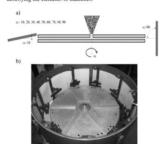
Fig. 2. Scheme of principle of operation (a) and the view of the chamber measuring Tribotester 9-Bitter (b) [7]
