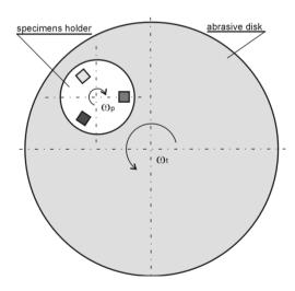
Fig. 5. Scheme of principle of operation of tribotester 3-POD
