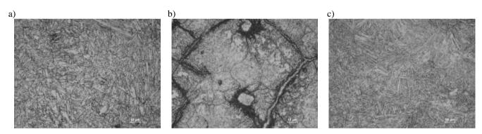
Fig. 1. The metallographic structures of studied cast steels and standard steel: a) low alloy cast steel - K2a; b) chromium cast steel - T2a; c) low alloy steel CREUSABRO®8000 - C8
