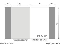
Fig. 3. Set of specimens fixed in the holder
