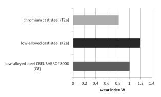
Fig. 11. Abrasive wear index W of studied materials in the tribological arrangement pin-abrasive disc
