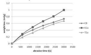
Fig. 9. Wear abrasive of cast steels K2a and T2a and steel C8
