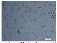
structure for DTA-C tester (high cooling rate) structure for DTA-Is tester (low cooling rate)
