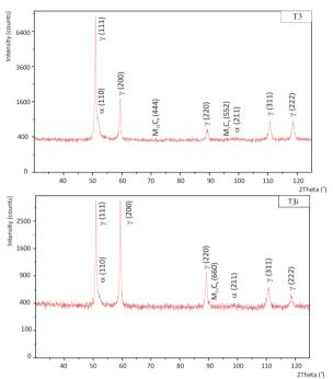
Fig. 5. X-ray diffractions pattern for chromium cast steel T3 by low and high cooling rates
