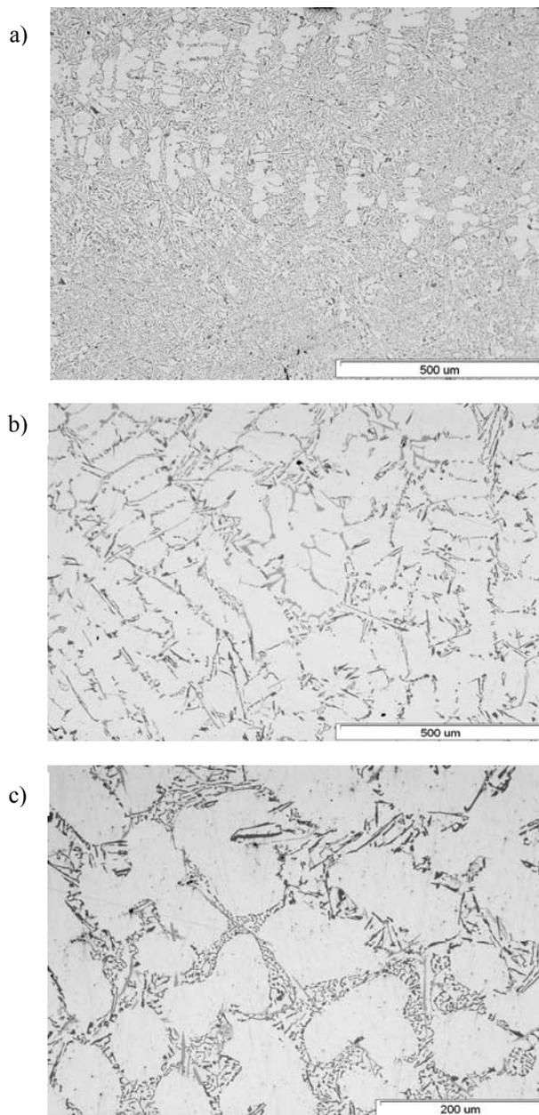
Fig. 3. Microstructure after modified AlSr10 alloy: a) AlSi3 silumin; b) AlSi6 and c) AlSi9 silumin
