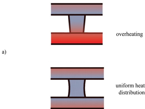
Fig. 3. Construction of ventilating element, a) improper; b) correct
