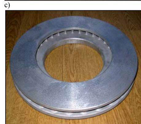
Fig. 6. Brake disc test castings; a) and b) rough castings, c) and d) after machining. a) and c) composite  $AlSi12Cu2Fe-(CrC14)_p$ , b) and d)  $AlSi11-(CrFe25C10)_p$
