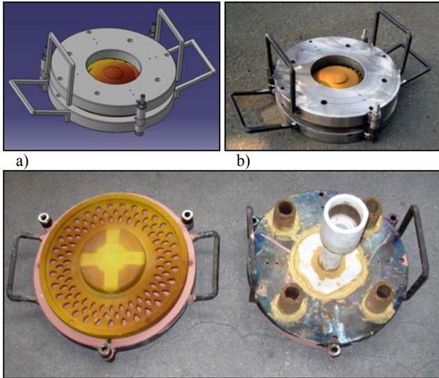
Fig. 5. Permanent mould for ventilated brake disc casting: a) Virtual model, b) real mould, c) mould with the gating system and the sand core
