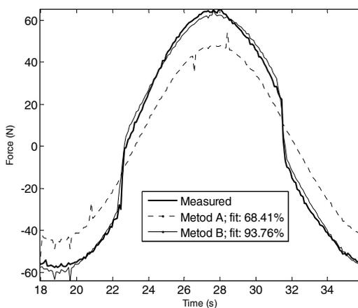
Fig. 5. Adjustment results for two parameters present in the friction model (test velocity  $v=0.018$  m/s)
