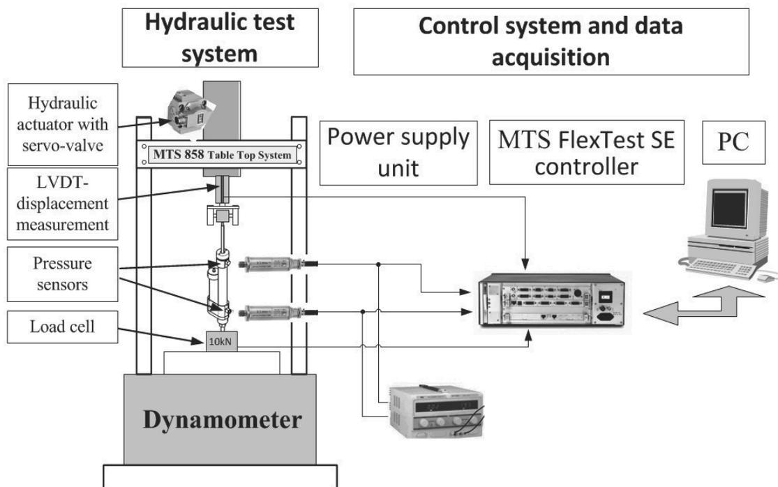
Fig. 3. Hydraulic damper and other components of the experimental setup
