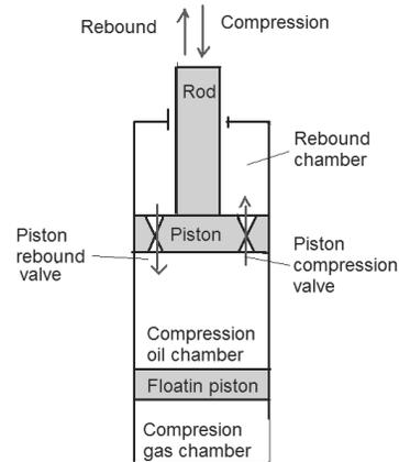
Fig. 1. Hydraulic damper scheme.
