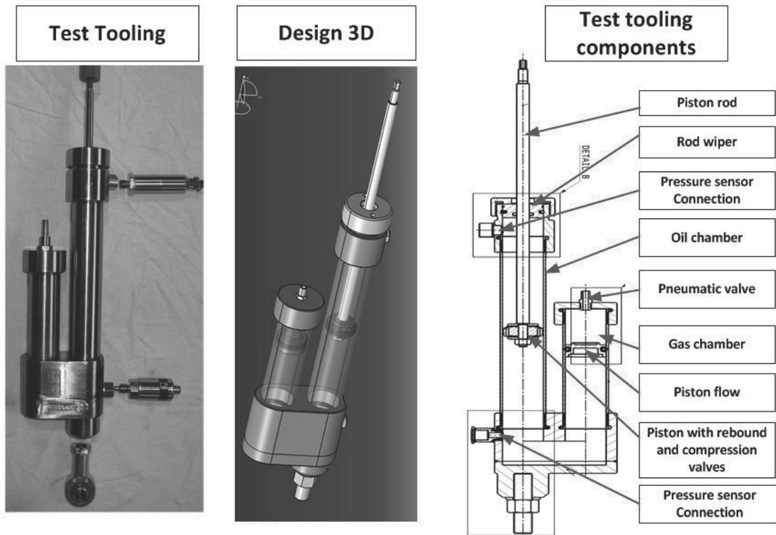
Fig. 2. Hydraulic test experimental setup
