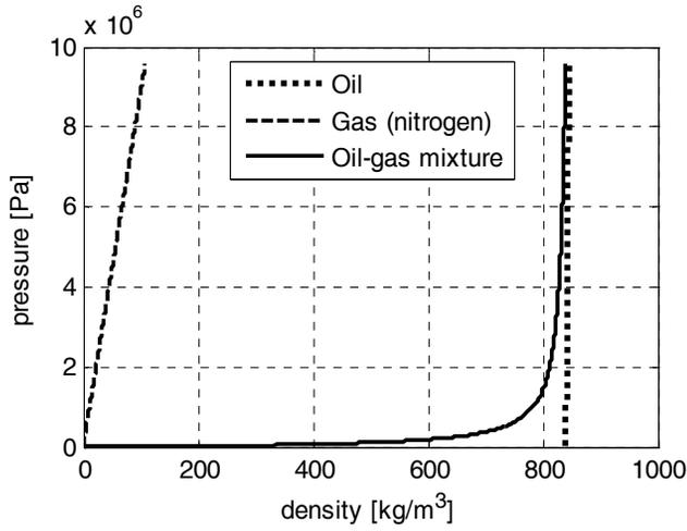
Fig. 4. Density-pressure relation for gas (isothermal), oil, and gas-oil mixture
