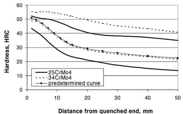
Fig. 2. Comparison of the predetermined Jominy curve and range of hardness change accepted as a model (34CrMo4) and suggested by the neural network (25CrMo4)
