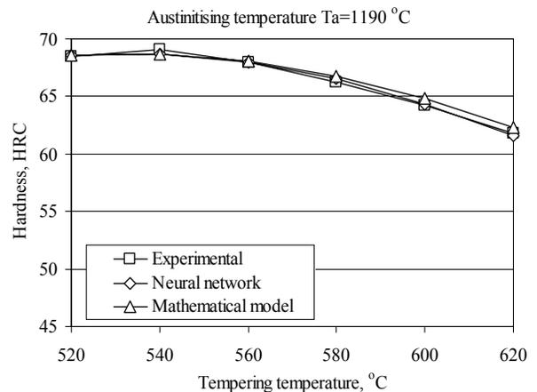
Fig. 6. Comparison of experimental results and hardness calculations for HS2-9-1-8 steel
