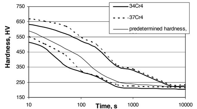
Fig. 5. Comparison of the predetermined hardness curve and range of hardness change accepted as a model (34Cr4) and suggested by the neural network (37Cr4)
