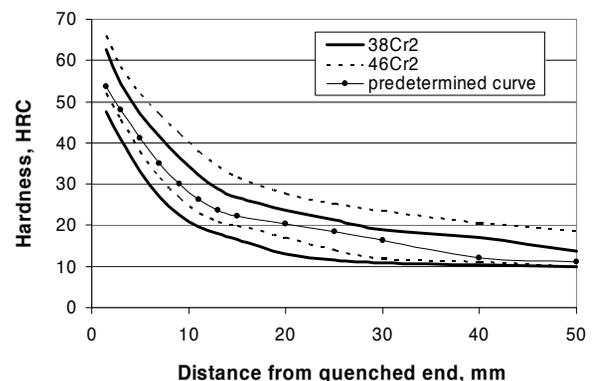
Fig. 3. Comparison of the predetermined Jominy curve and hardness ranges for steel grades suggested by the neural network: variant 1-38Cr2; variant 2 - 46Cr2
