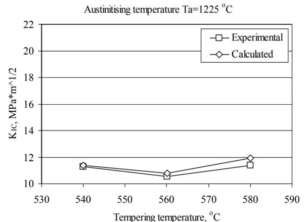
Fig. 7. Comparison of the calculated  $K_{Ic}$  coefficient with the experimental data for HS6-5-2 steel
