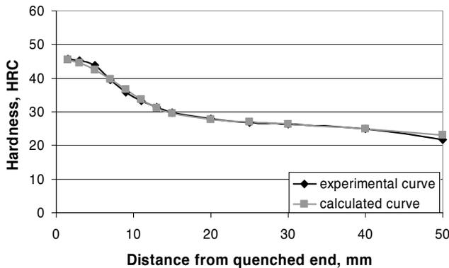
Fig. 1. The comparison of the experimental and calculated curves for the steels with a mass concentration of elements: 0.19% C, 0.94% Mn, 0.28% Si, 0.94% Cr, 0.17% Ni, 0.23% Mo
