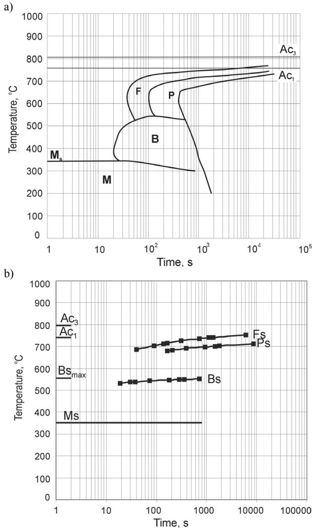
Fig. 4. CCT diagram for steel with concentrations: 0.36% C, 0.49% Mn, 0.25% Si, 1.54% Cr, 0.21% Ni, austenitised at temperature of 860°C: a) experimental, b) calculated
