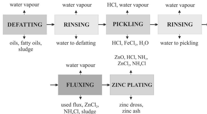
Fig. 3. Schema of the process flow of the zinc plating technological process
