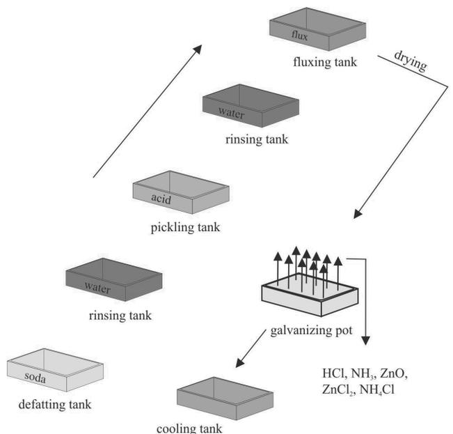
Fig. 2. Schema of the zinc plating technological process [16]
