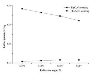
Fig. 26. Comparison of the change of lattice parameter estimated for Ti(C,N) and (Ti,Al)N coating
