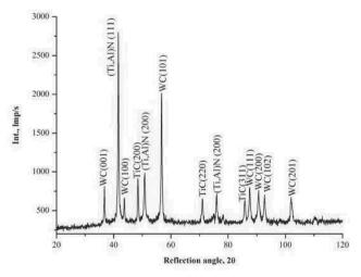
Fig. 20. X-ray phase analysis of the (Ti,Al)N coating (Bragg-Brentano geometry)
