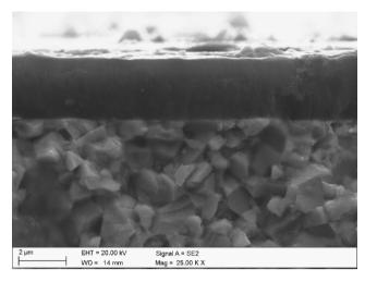
Fig. 6. Fracture surface of the gradient (Ti,Al)N coating deposited onto the cemented carbides substrate
