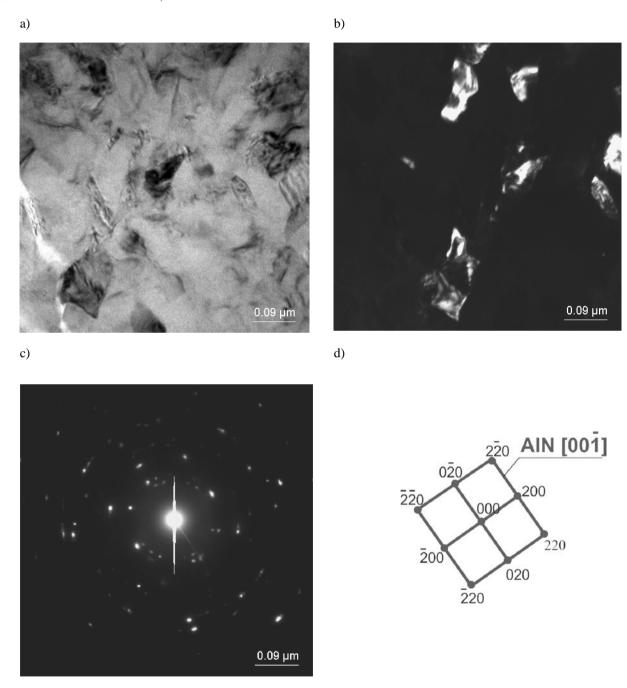
Fig. 14. Structure of (Ti,Al)N coating: a) bright field; b) dark field from ( $\overline{200}$ ) AlN reflex; c) diffraction pattern from area b and d) solution of the diffraction pattern
