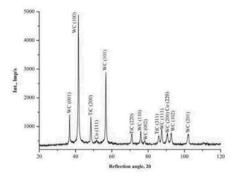
Fig. 19. X-ray phase analysis of the cemented carbides substrate (Bragg-Brentano geometry)
