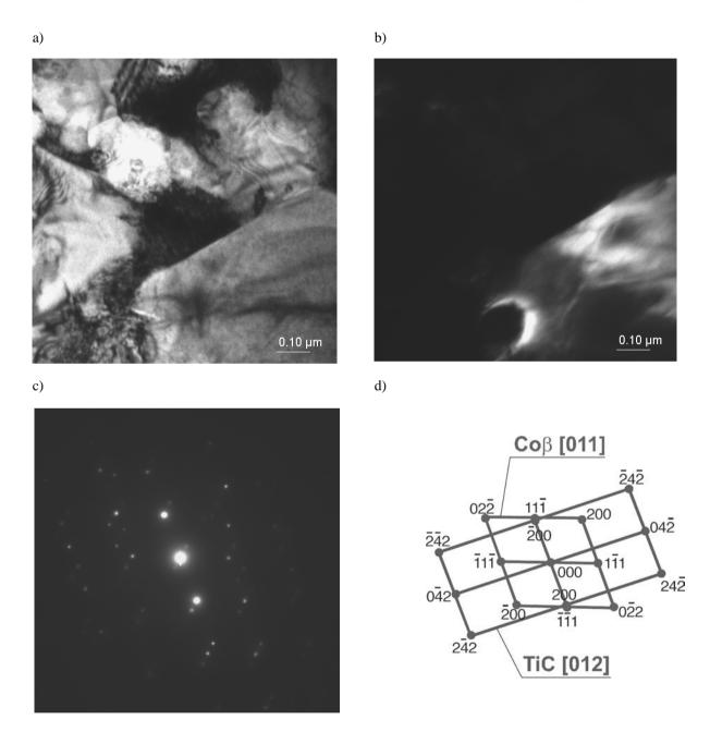
Fig. 12. Structure of cermet substrate: a) bright field; b) dark field from  $(\overline{2}00)$  TiC i  $(11\overline{1})$  Co reflex; c) diffraction pattern from area b and d) solution of the diffraction pattern
