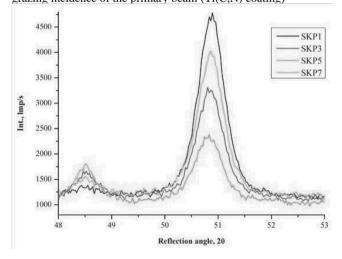
Fig. 25. Change of (200) reflection's position in relation to grazing incidence of the primary beam ((Ti,Al)N coating)
