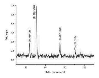
Fig. 22. X-ray phase analysis of the (Ti,Al)N coating (grazing incidence X-ray diffraction GIXRD method),  $\alpha$ =1
