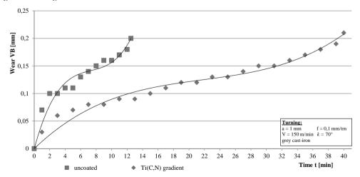
Fig. 38. Comparison of the approximated values of the VB wear of the  $Al_2O_3+TiC$  oxide tool ceramics sample: uncoated and coated with the Ti(C,N) gradient coating, depending on machining time
