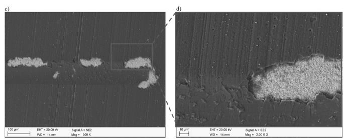
Fig. 32. a,b,c,d) Characteristic failure obtained by scratch test of the (Ti,Al)N coating deposited on cemented carbides substrate
