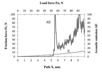
Fig. 30. a) Indenter trace with the optical  $L_c$ =45N load (mag. 200x), b) scratch test results of the (Ti,Al)N coating surface deposited on cemented carbides substrate
