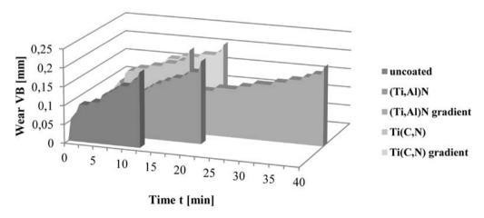
Fig. 35. Comparison of the approximated values of the VB wear of the  $Al_2O_3+TiC$  oxide tool ceramics sample: uncoated and coated with the PVD coatings, depending on machining time
