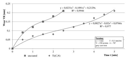
Fig. 37. Comparison of the approximated values of the VB wear of the cemented carbides sample: uncoated and coated with the Ti(C,N) coating, depending on machining time
