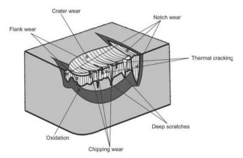
Fig. 3. Tool wear model [1,65]
