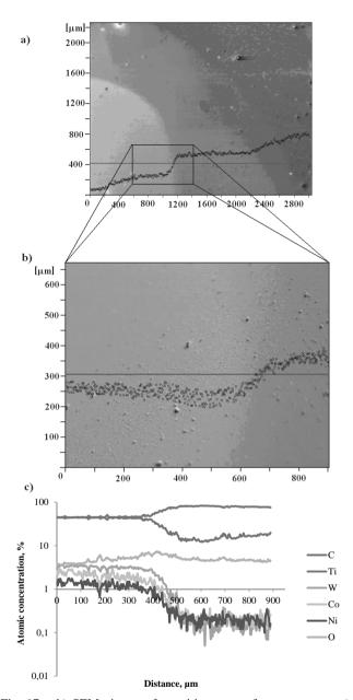
Fig. 17. a,b) SEM picture of transition zone of sputter crater, c) line profile of chemical composition (AES) of gradient Ti(C,N) coating on cermet substrate
