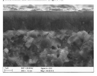
Fig. 8. Fracture surface of the gradient Ti(C,N) coating deposited onto the cermet substrate
