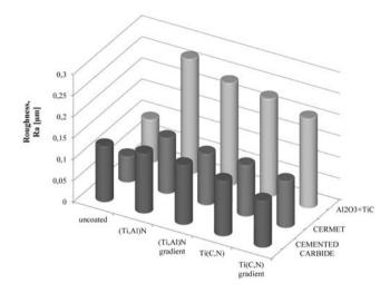
Fig. 27. Comparison of the roughness parameter  $R_{\text{a}}$  of the investigated materials
