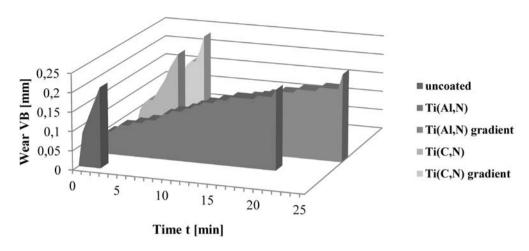
Fig. 33. Comparison of the approximated values of the VB wear of the cemented carbides sample: uncoated and coated with the PVD coatings, depending on machining time
