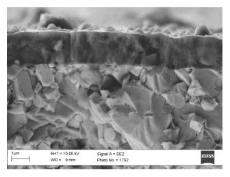
Fig. 5. Fracture surface of the (Ti,Al)N coating deposited onto the cemented carbides substrate
