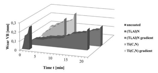
Fig. 34. Comparison of the approximated values of the VB wear of the cermets sample: uncoated and coated with the PVD coatings, depending on machining time
