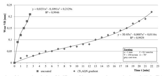
Fig. 36. Comparison of the approximated values of the VB wear of the cermets sample: uncoated and coated with the (Ti,Al)N gradient coating, depending on machining time
