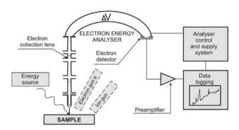
Fig. 2. Schematic diagram of X-Ray Photoelectron Spectroscopy (XPS)
