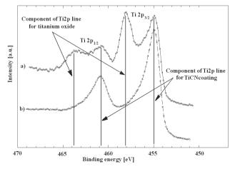
Fig. 16. The shape of Ti2p lines obtained by XPS method for  ${\rm Ti}(C,N)$  coating: a) "fresh" ex situ surfaces, b) after sputtering  ${\rm Ar}^+$  ions for t=4min
