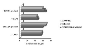
Fig. 29. Comparison of the critical load according to the scratch test of the investigated coating deposited onto cemented carbides, cermets and  ${\rm Al}_2{\rm O}_3$  type oxide tool ceramics
