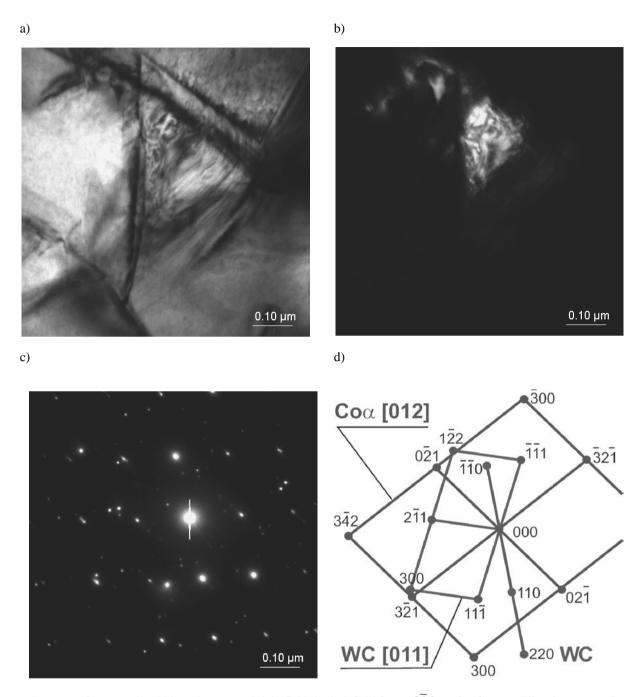
Fig. 11. Structure of cemented carbides substrate: a) bright field; b) dark field from  $(2\overline{I}I)$  WC reflex; c) diffraction pattern from area b and d) solution of the diffraction pattern
