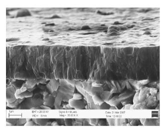
Fig. 7. Fracture surface of the (Ti,Al)N coating deposited onto the cermet substrate
