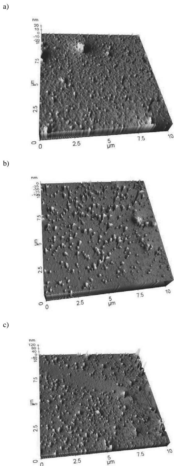
Fig. 6. The AFM topography image of the surface thin film of polymer Oxp-Per-6F (3:1:2) coated with a spin speed: a) 1000 rev / min, b) 2000 rev / min, c) 3000 rev / min
