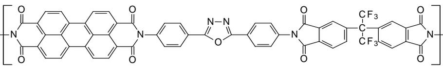
Polyoxadiazoles belong to a group of conductive polymers that can be used in photovoltaic and optoelectronics. Responsible for the transport of electrons is a system of conjugated double bonds of the polymer chain. Representative of this group is shown on Figure 1. Polyoxadiazoles characterized by their high performance of electrical and optical properties, good hydrolytic stability, highly ordered systems, mechanical resistance and high thermal stability [8,9].
