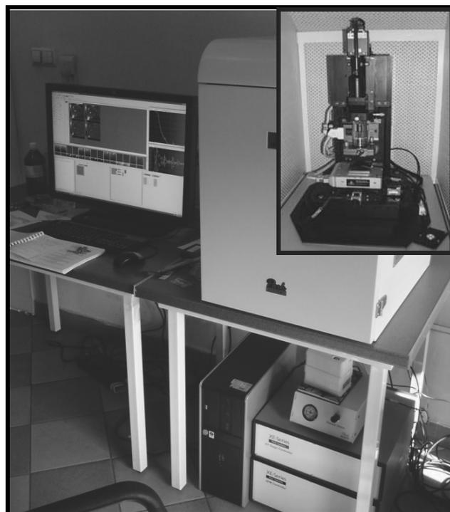
Fig. 2. The position measuring AFM microscope in the laboratory of the Institute of Engineering Materials and Biomaterials, Silesian University of Technology
