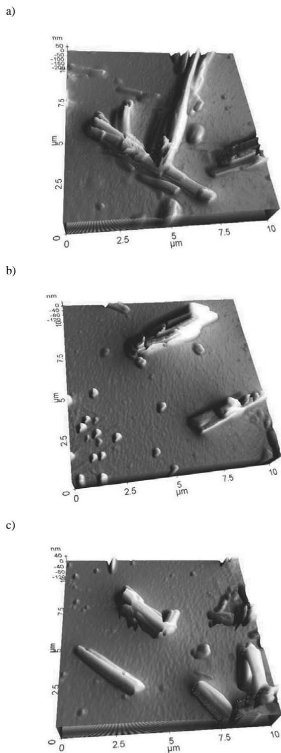
Fig. 5. The AFM topography image of the surface thin film of polymer Ox-Per-6F (2:1:1) coated with a spin speed: a) 1000 rev / min, b) 2000 rev / min, c) 3000 rev / min
