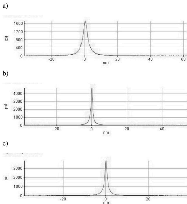
Fig. 10. The histogram of frequency of the occur height for a thin film of polymer Oxp-Per-6F (2:1:1) coated with a spin speed at: a) 1000 rev / min, b) 2000 rev / min, c) 3000 rev / min
