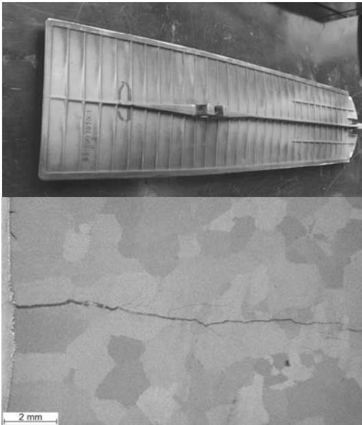
Fig. 1. View and macrostructure of a crack of jet engine inner flap made of nickel superalloy ZS-3DK (ЖС-3ДК)
