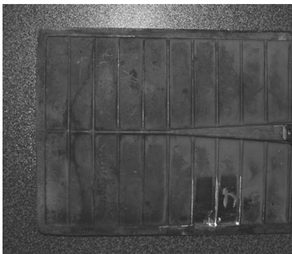
Fig. 8. View of a repaired crack from the inner flap of nickel superalloy ZS-3DK (ЖС-3ДК), using HPDL laser welding, Table 4
