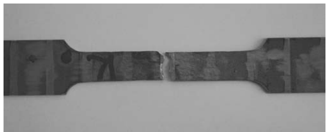
Break in the HAZ
