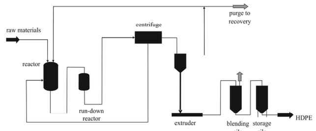
Fig. 1. Flow diagram of an HDPE production [13]
