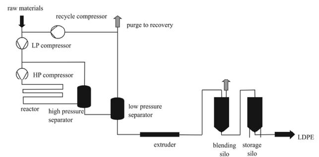
Fig. 2. Flow diagram showing LDPE production [13]
